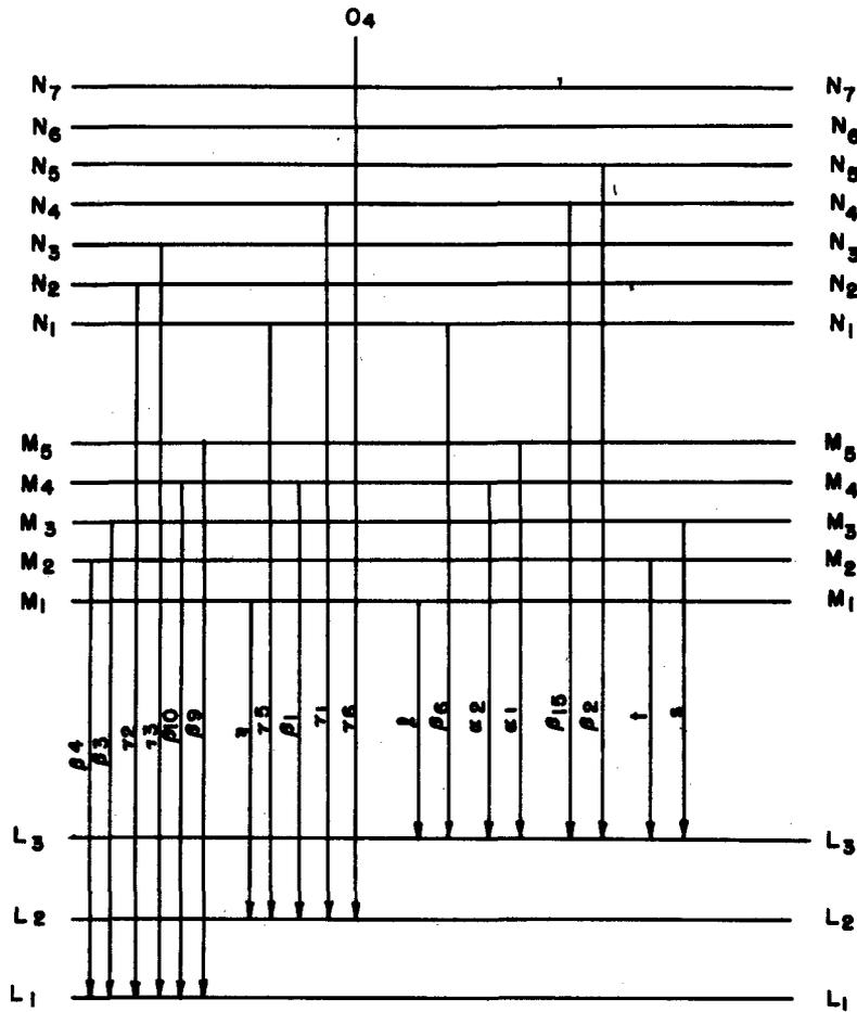
Fig. 3. Diagram of L x-ray nomenclature
