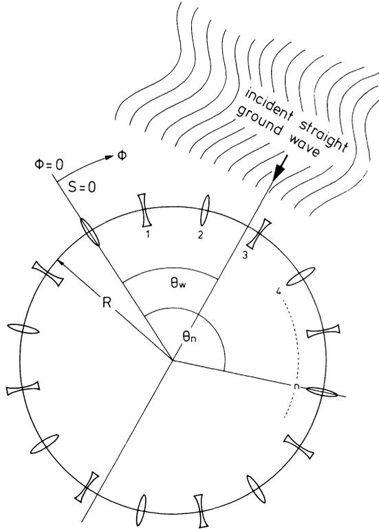
FIGURE 2 Sketch of geometry as described by the model and nomenclature.
