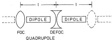
FIGURE 1 Sketch of a simple FODO cell as used in the model.
