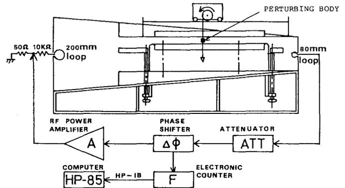
Fig. 4. Block diagram of the system used to measure field distributions in the gap.
