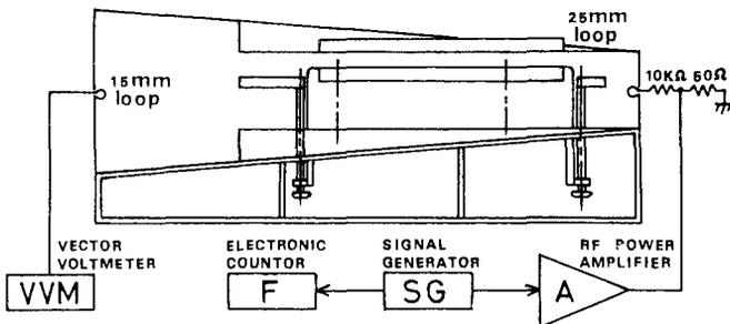
Fig. 6. Circuit used for measurement of Q-values.
