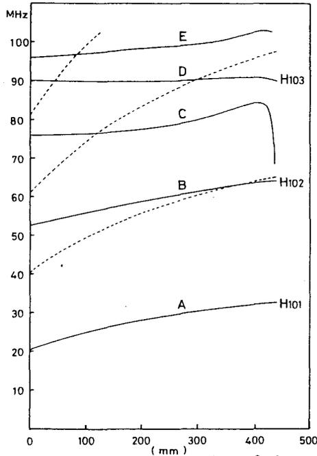
Fig. 2. Resonance frequencies of the cavity vs. position of the tuning plate.
