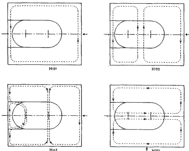
Fig. 3. Various modes of resonance. Broken lines show magnetic flux. Arrows indicate positions of coupling with which the cavity is excited.
