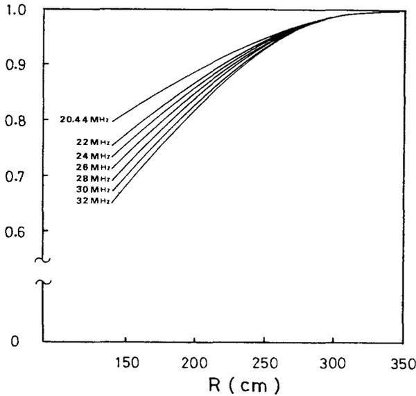
Fig. 5. Voltage distributions along acceleration gap. Values are normalized at the extraction radius.
