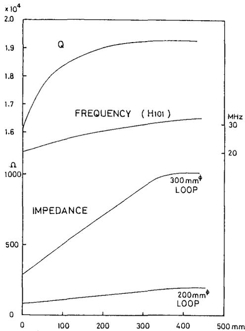
Fig. 7. Measured Q-values and input impedances of the cavity.
