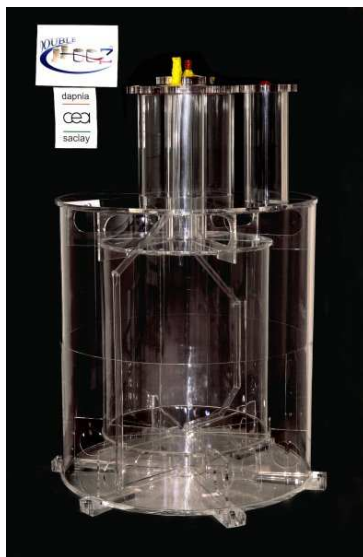
Fig. 3. Double acrylic vessel of the Double Chooz 1/5 mock-up.
