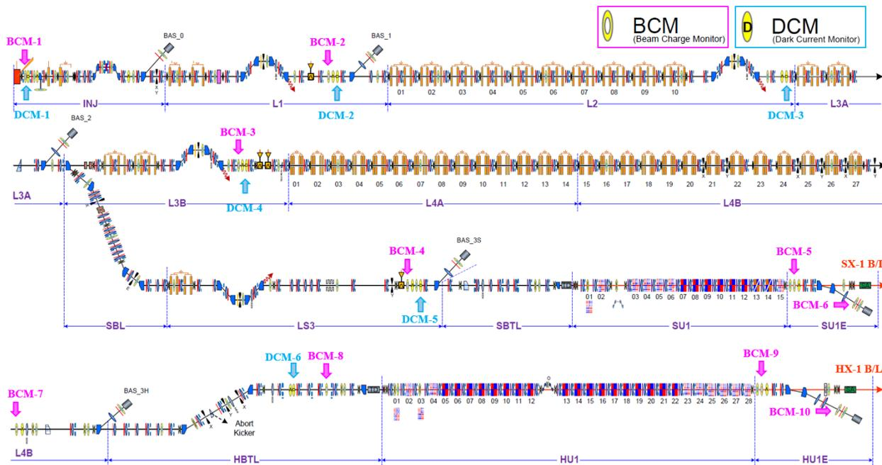
Figure 8: Installation position of Turbo-ICT & DCM.
