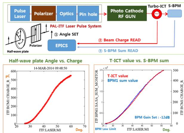
Figure 2: Generation of the laser cathode gun and results of measurement of charge.
