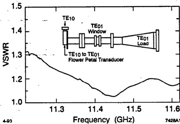
Figure 6. Measured rf match and schematic of combined TE<sub>10</sub> to TE<sub>01</sub> transducer and TE<sub>01</sub> disk window with matched termination.
