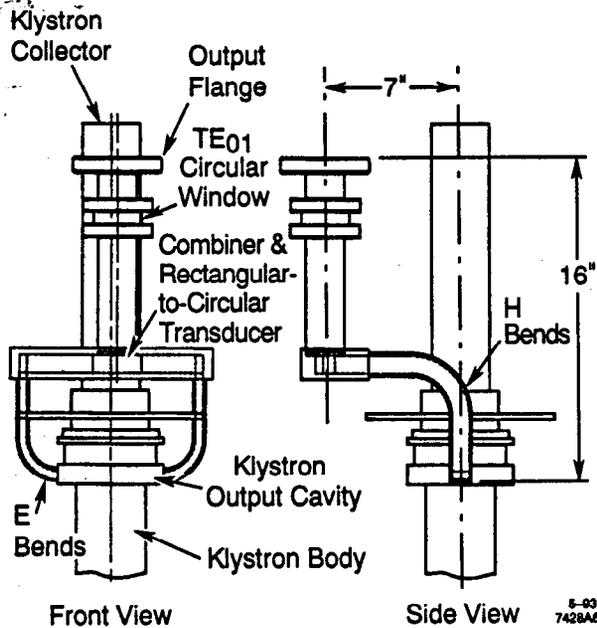
Figure 5. Arrangement of waveguides used to obtain TE<sub>01</sub> circular waveguide output.
