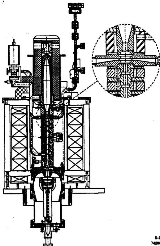
Figure 1. Assembly drawing of XC8 in focusing coil.
