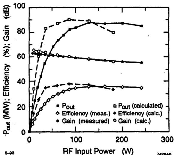
Figure 4. Comparison of computed and measured performance of XC6—two uncoupled output cavities (200 ns pulses, 60 pps).
