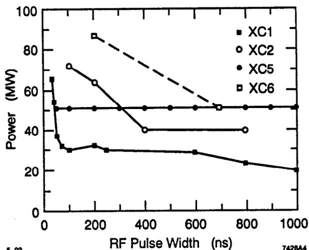
Figure 3. Effect of pulse width on achievable peak power.
