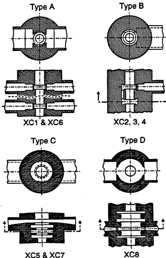
Figure 2. Five types of output circuits tested by SLAC in XC series.
