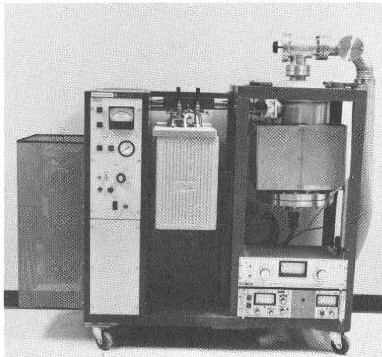
Fig. 12. Portable, contaminant-free roughing system showing the oilless vacuum pump on the left, the sorption pump in the center, and the titanium sublimator on the right.
