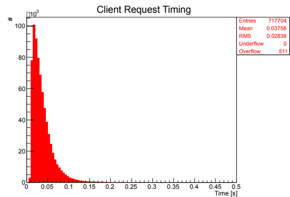
Figure 9. The client request timing using PycURL to connect to the server.10 threads are accessing cmsweb-testbed in parallel.
