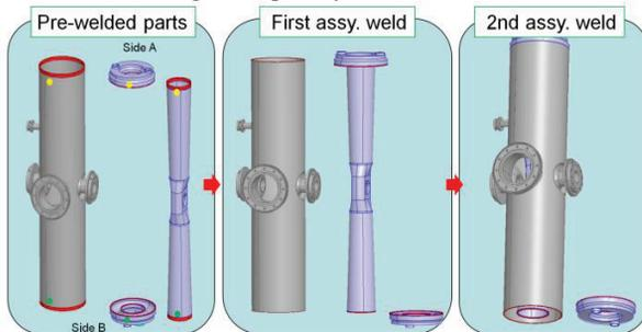
Figure 3: Intermediate HWR configurations for RF frequency tuning by trimming operations.
