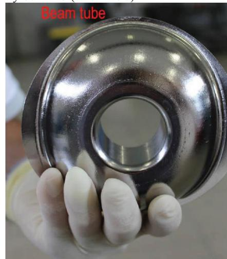
Figure 1: beam port of the HWR.
