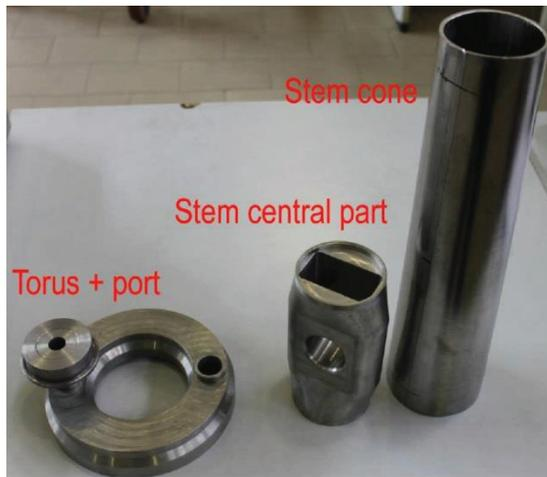
Figure 2: Nb parts of the pre-series HWR.
