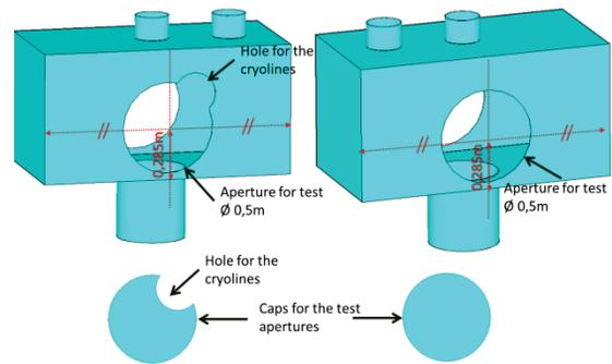
Figure 16: Magnetic shields apertures and caps.
