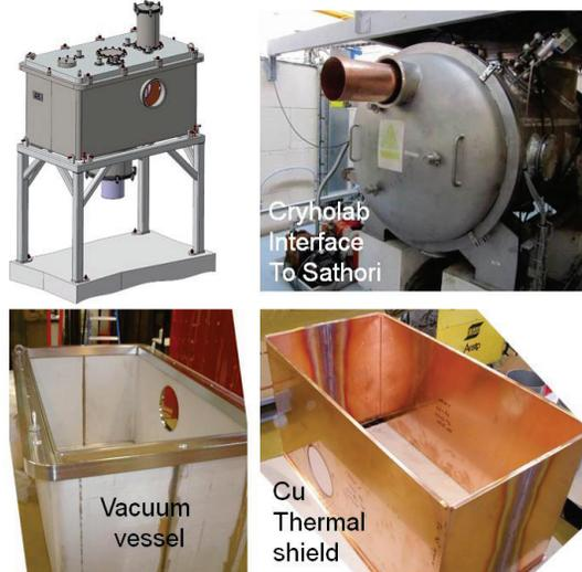
Figure 14: Manufacturing of Sathori components.
