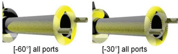
Figure 9: The  $-60^\circ$  jet improves of the torus coverage.
