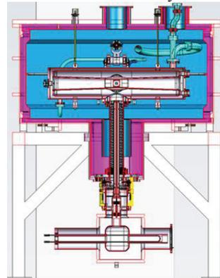
Figure 13: Cut view of Sathori equipped with HWR, tuner and FPC.
