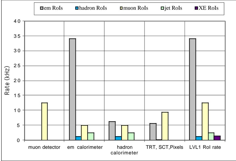
Figure 3. RoI rates (kHz), high luminosity, 39.4 kHz LVL1 rate, sequential processing
