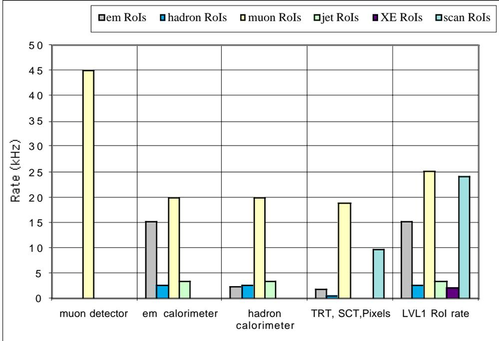
Figure 2. RoI rates (kHz), low luminosity, 40.1 kHz LVL1 rate, sequential processing
