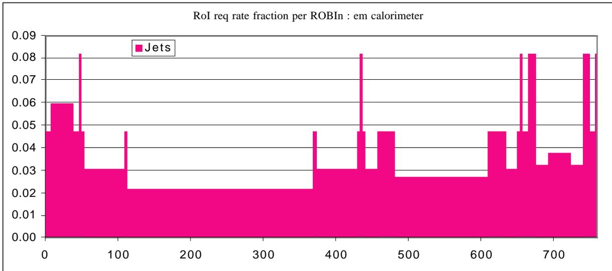
Figure 24. RoI request rate fraction per em calorimeter ROBIN for jet RoIs
