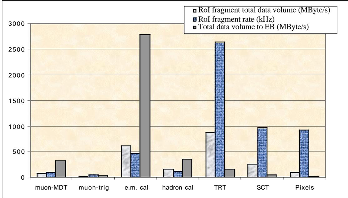
Figure 4. Low luminosity, 40.1 kHz LVL1 rate, sequential processing, B-physics trigger. The RoI fragment rate is the total rate into the LVL2 processors
