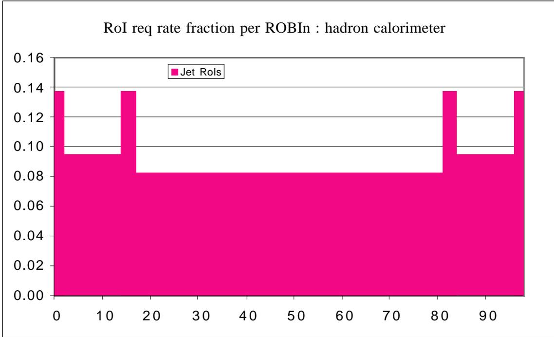
Figure 27. RoI request rate fraction per hadron calorimeter ROBIN for jet RoIs
