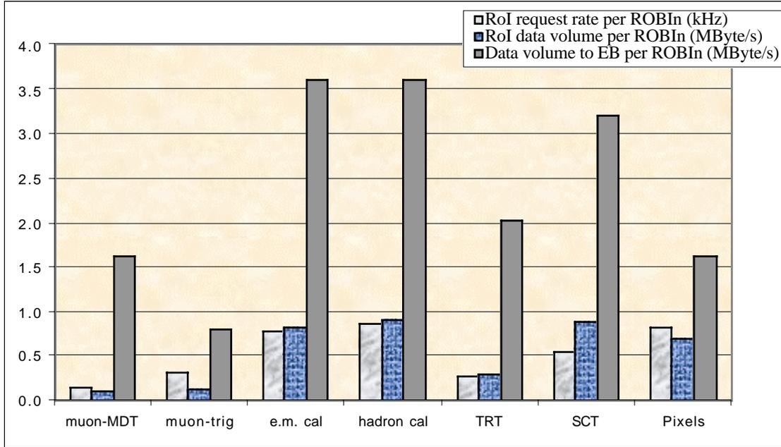
Figure 7. High luminosity, 39.4 kHz LVL1 rate, sequential processing
