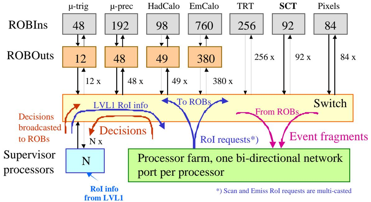
Figure 1. System architecture : baseline model.
