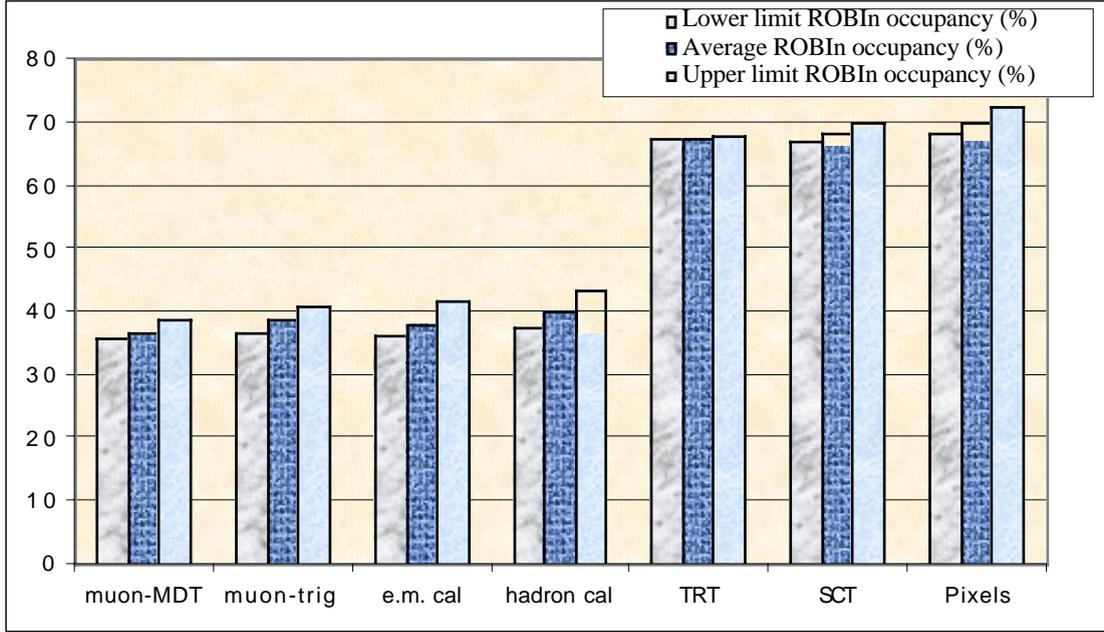
Figure 14. Low luminosity, nominal LVL1 rate, sequential processing, B-physics trigger
