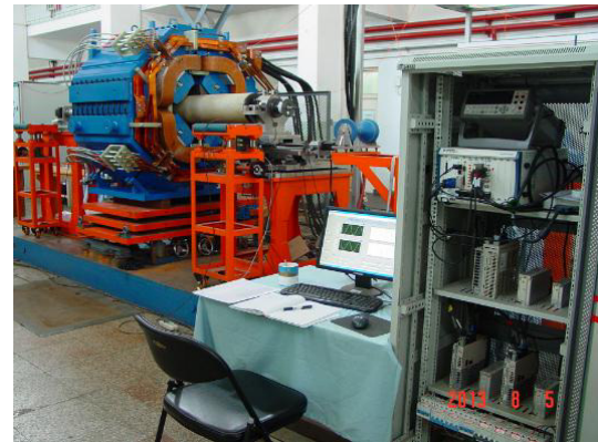
Figure 1: Quadrupole and Setup of the Rotating Coil.
