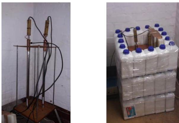
Fig5. Setup used in Freiberg (Germany) in Reiche Zeche shaft Left: Bare counters for the first phase measurements. Right: Counters in borax shield for the second phase measurements.
