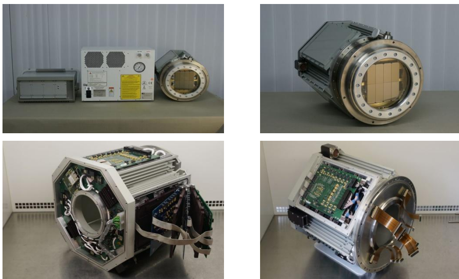
Fig10. Technical groundwork for TNRT: photodetector with a mosaic sensor
