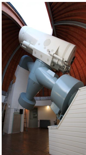
Fig4. The complex for studying fast variability in the BTA Nasmyth-1 (N-1) focus. N-1: a complex in “hot standby”: it will operate in the second half of 2018. Can be started up during several minutes. It includes the EM CCD with the temporal resolution till 1 msec. Performance capabilities: wide-band photometry and polarimetry.
