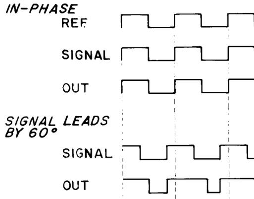
Fig. 4. Desired phase detector outputs before integration.
