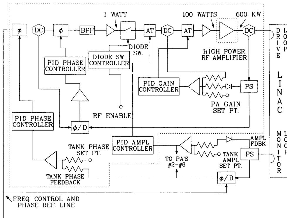
Fig. 1. A single rf amplifier chain.
