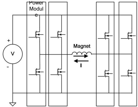
Figure 4 Power Modules Arranged for Bipolar Output
