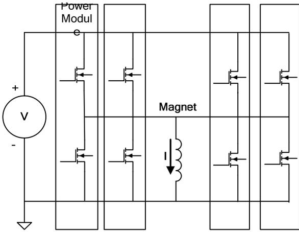
Figure 3 Power Modules Arranged for Unipolar Output
