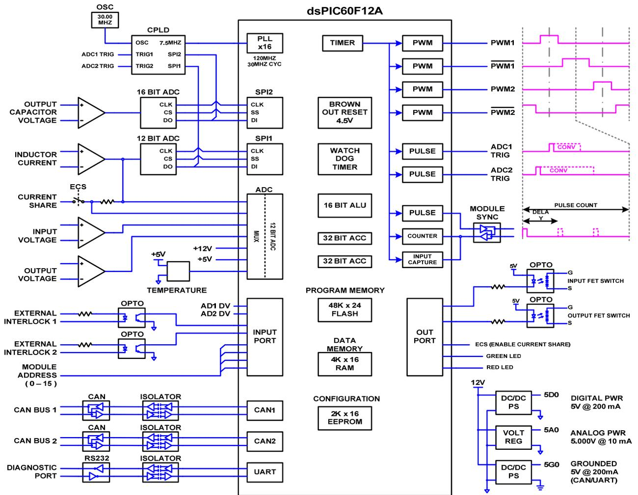
Figure 5 Controller Block Diagram
