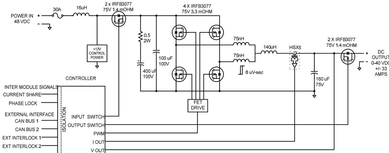
Figure 2 Power Module Schematic Diagram
