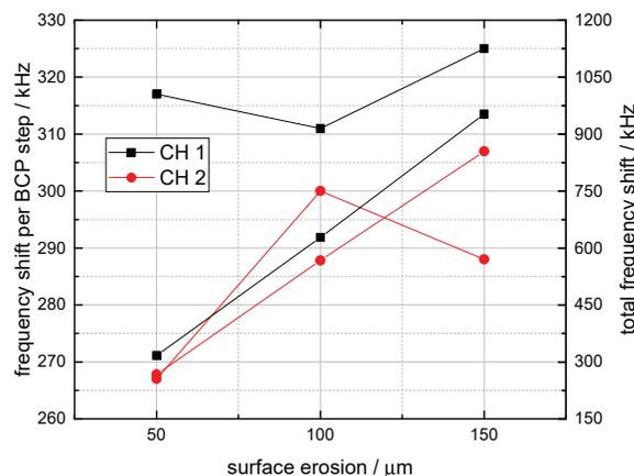
Figure 3: Frequency change for each 50  $\mu\text{m}$  BCP step as well as the total frequency change for CH 1 and CH 2.
