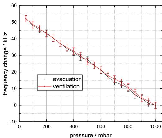
Figure 2: Pressure sensitivity of CH 2 during evacuation and ventilation.
