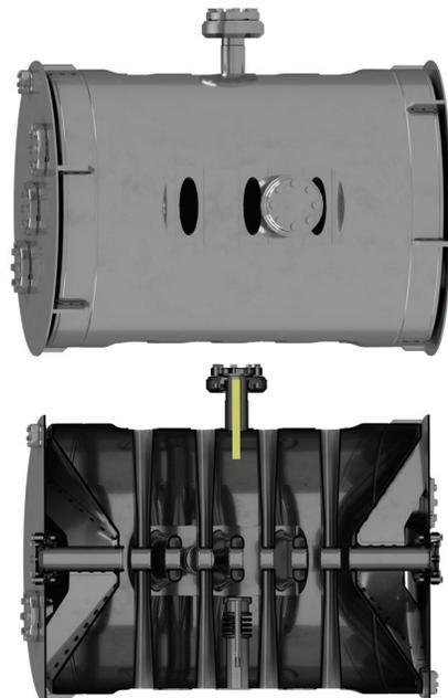
Figure 1: Layout of the SC 217 MHz CH-Cavity 2 and 3.
