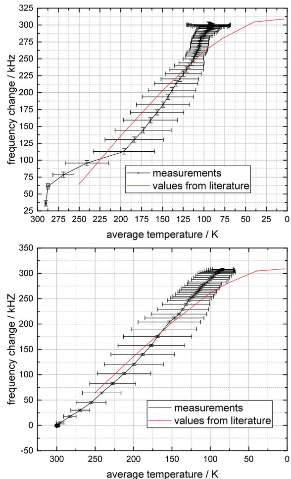
Figure 5: Frequency change depending on the average temperature of CH 1 (Top) and CH 2 (Bottom) during the preliminary cold test compared to [9].
