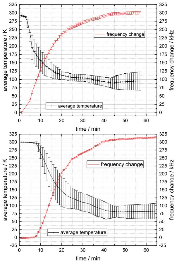
Figure 4: Resonance frequency and average temperature of CH 1 (Top) and CH 2 (Bottom) during the preliminary cold test.
