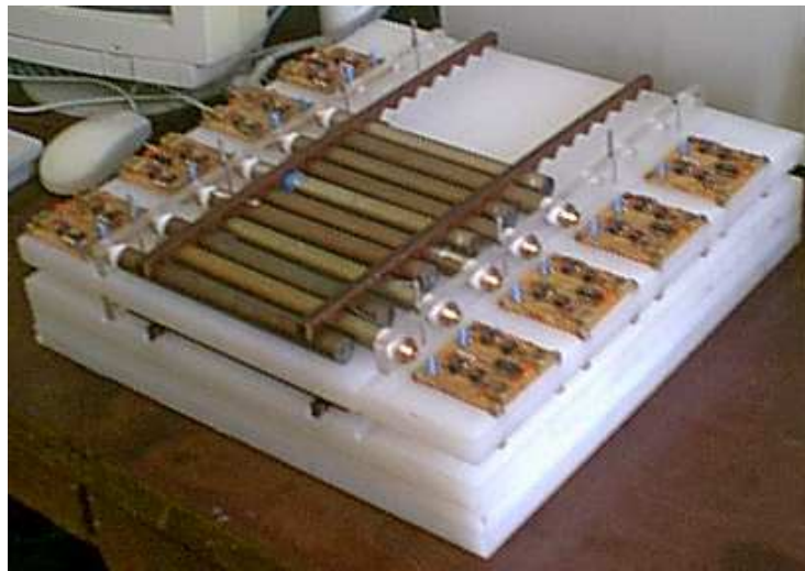
Figure 2.16: The neutron detector during the test and assembly phase. Some of the ^3\text{He} tubes, the polyethylene moderator and the electronic boards are visible.
