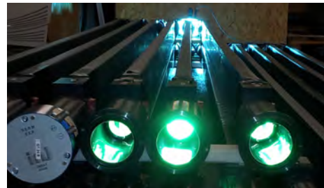
Figure 4.4: Hardening of the UV glue connecting light guide and scintillator.
