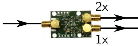
Figure 4.9: Labelled photograph of the A nalogue f an-out A mplifier board (short: ‘AfA’) which features one input and two outputs, one of them with a gain of 1 and one with a gain of 2. Picture courtesy by F. Messi.
