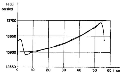
Fig. 3 Average magnetic field vs. radius for  $N = 6$ .
