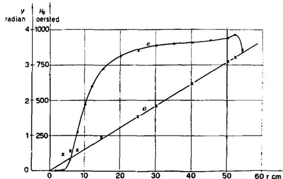
Fig. 8 a) Amplitude of the magnetic field 6th harmonic  $H_6$  vs. radius; b) The 6th harmonic phase vs. radius.
