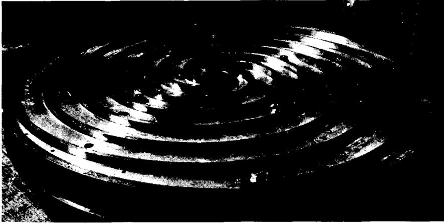
Fig. 6 Pole piece with spiral shims for  $N = 4$ .
