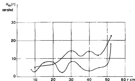
**Fig. 10** Amplitudes of the low harmonics of the magnetic field vs. radius for  $N = 6$  (—○—○— first harmonic, —×—×— second one).
