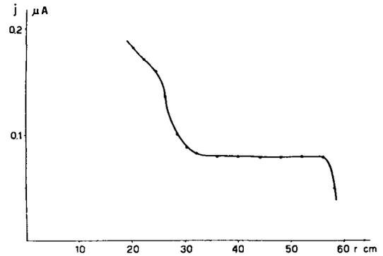
Fig. 4 Beam current at different radii ( $V_0 = 11$  kV).
