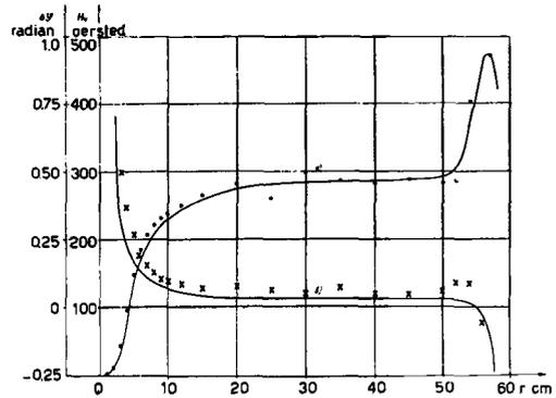
Fig. 7 a) Amplitude of the fourth harmonic of the magnetic field vs. radius, b) Deviation of the 4th harmonic phase from the spiral.
