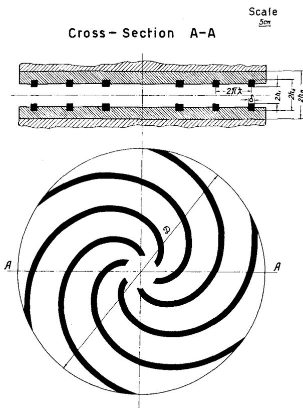
Fig. 9 Pole piece with spiral shims for  $N = 6$  (diagram).
