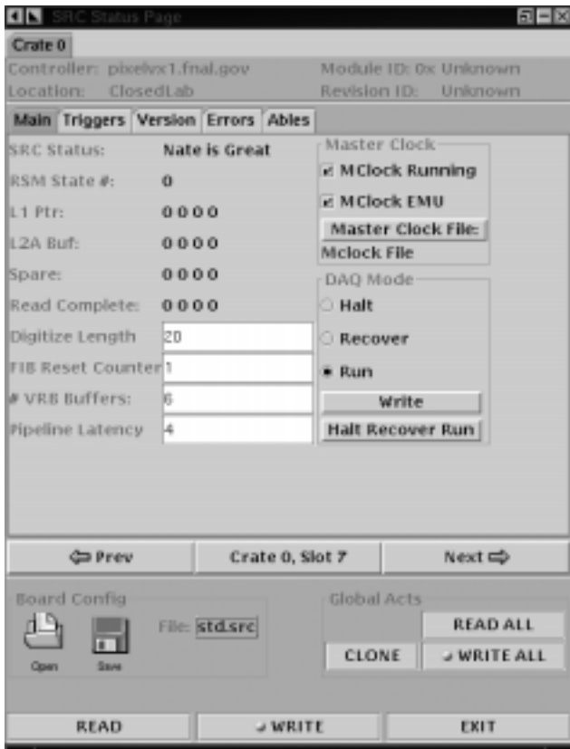
Figure 3. Board Display. The board specific details are encapsulated within a standard frame, which includes navigation between boards and transference of the state between the GUI, hardware, and static storage.
