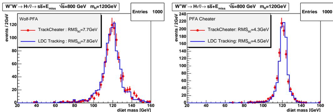
Figure 2: The di-jet mass distribution in the sample of the  $e^+e^- \rightarrow W^+W^-\nu\bar{\nu} \rightarrow H\nu\bar{\nu}$  events. Left plot shows results obtained with the realistic Particle Flow Algorithm Wolf-PFA. Right plot - with the perfect PFA. Dots with error bars correspond to the runs with the perfect tracking, solid histograms - with the realistic LDC tracking.
