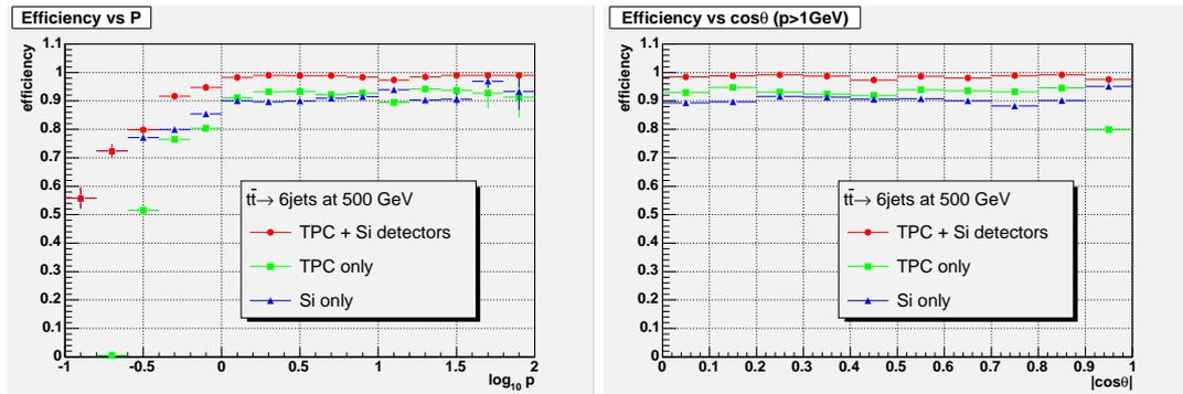
Figure 1: The track finding efficiency as a function of the track momentum (left plot) and polar angle (right plot) in the sample of the  $e^+e^- \rightarrow t\bar{t}$  events at 500 GeV. The dependence of the track efficiency on the polar angle is presented only for tracks with momentum greater than 1 GeV.
