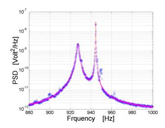
Figure 3: The measured Power Spectral Density (PSD) of the SQUID amplifier output. The fitting function (continuous line) is given in eq.1. When the readout is at liquid helium te fit estimates  $T = 4.2 \pm 0.4$  K, in agreement with the thermodynamic temperature.
