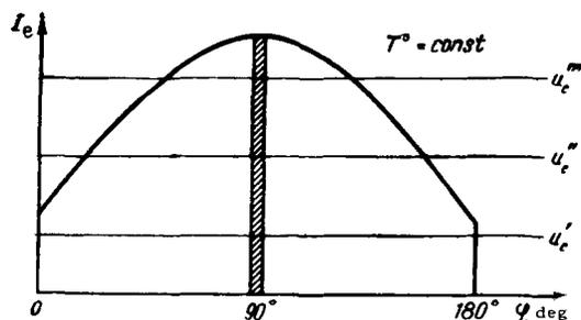
Figure 1. Dependence of cathode emission current on the phase of the rf field of the resonator. The straight lines  $u_c = \text{const}$  indicate the action of positive bias.
