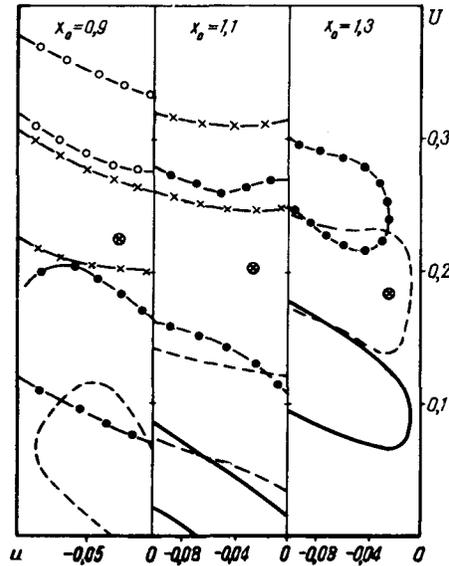
Figure 2. Capture regions according to initial phases, angles and energies, for different positions of the cathode along the resonator axis:
