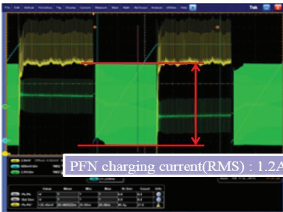
Figure 5: PFN charging current.
