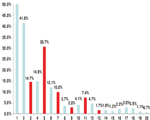
Figure 10: Harmonic current spectrum measured from AC 480 V.
