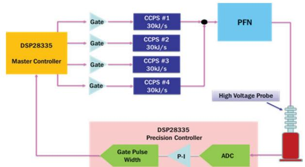
Figure 3: CCPS precision control configuration.
