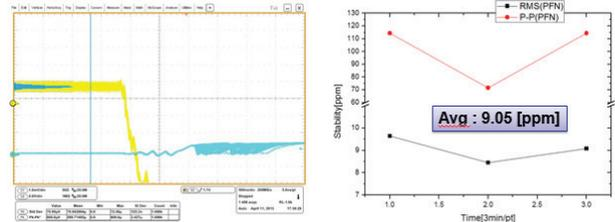
Figure 7: PFN voltage stability measurement.
