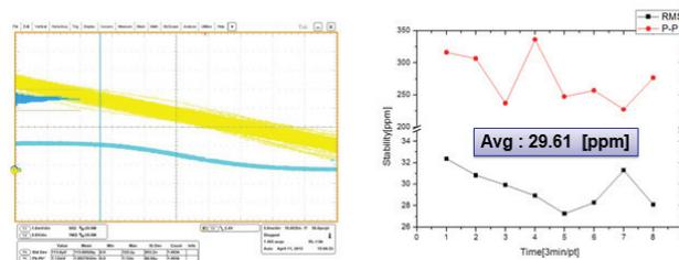
Figure 8: Beam voltage stability measurement.
