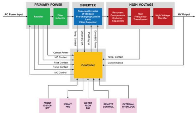
Figure 2: Block diagram of the inverter power supply.
