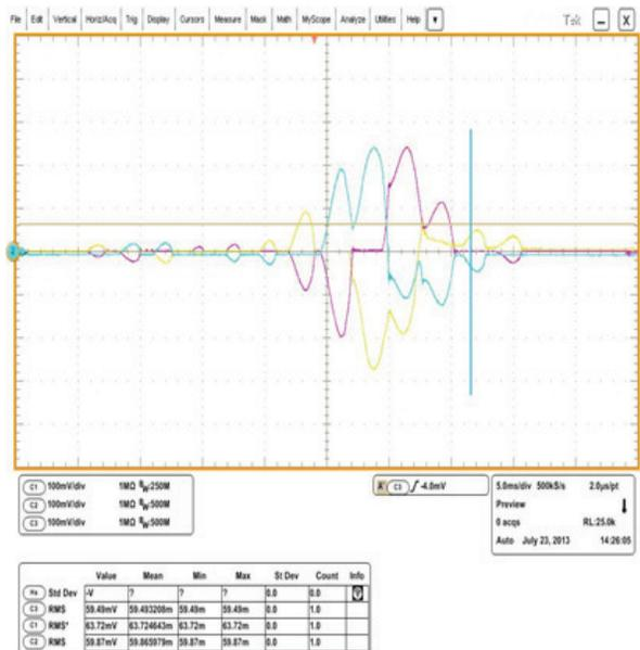
Figure 9: Current waveforms from AC 480 V.
