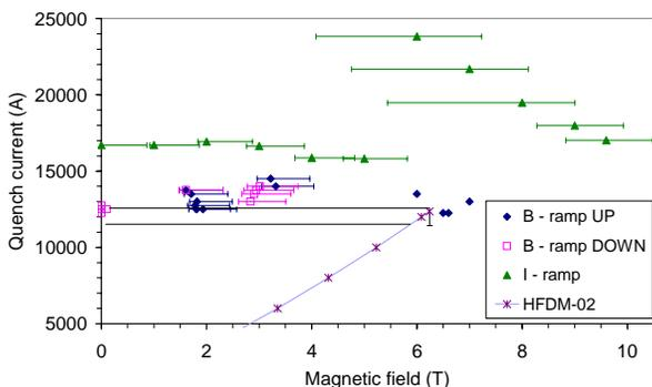
Fig. 6. MJR-sample B-ramp results compared with I-ramp quenches and HFDM02 performance at 4.3 K
