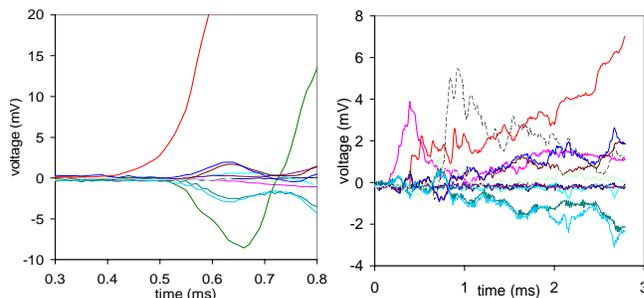
Fig. 4. Voltage onset at beginning of a quench in the PIT-sample during test at 4.3 K with BG field = 7 T (left) and without BG field (right). The ramp rate was 150 A/s in both cases. Quench current was 29386 A (left) and 28575 A (right). Signals show the voltage on different segments.
