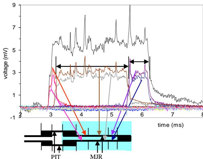
Fig. 8. Propagation of a spike along the whole MJR-sample (splices excluded) at 4.3 K, 1 T. The current was about 17 kA with a ramp rate of 150 A/s. The highest peak is 9 mV, and the time intervals shown are: 2.4 and 0.7 ms.
