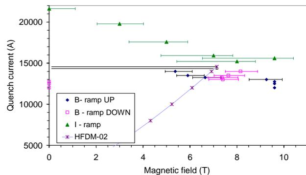
Fig. 7. MJR-sample B-ramp results at 1.9 K compared with I-ramp quenches at 1.9 K and HFDM02 performance at 2.2 K.
