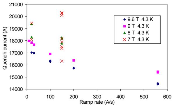
Fig. 5. Ramp rate dependence of the MJR-sample at 4.3 K test.
