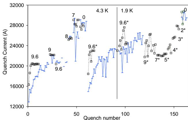
Fig. 2. Comparison of quench history during first (dash markers) and second test (square markers) of the PIT-sample. Numbers indicate the BG field during the second test.
