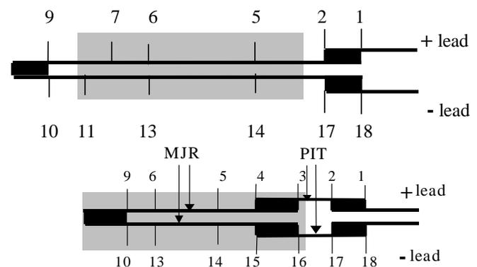
Fig. 1. From top to bottom, schematic of PIT-sample, and MJR-sample, showing cable and splice (black box) positions with respect to the external field (gray box). Numbers indicate voltage taps.
