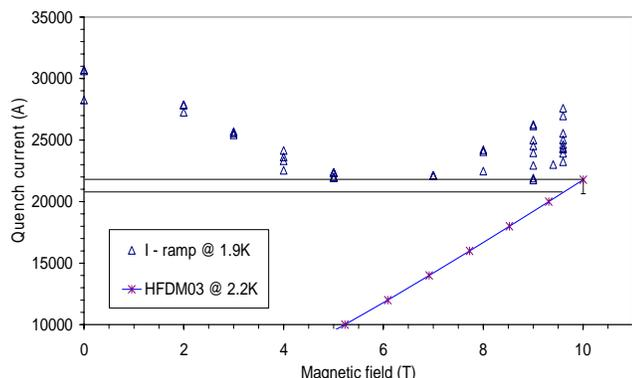
Fig. 3. Quench currents of the PIT-sample at 1.9 K as function of the BG field.
