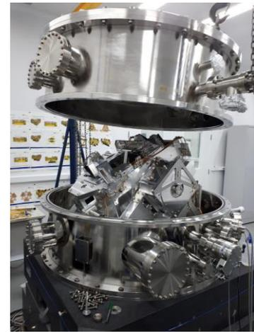
Figure 1: Overall view of the HD-DCM with its major subparts, namely: granite bench, double-side goniometric system, goniometer frame, long-stroke frame, 1<sup>st</sup> and 2<sup>nd</sup> modules, and the vacuum vessel. (For references, see [5].)
