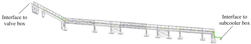
Fig. 9.15 Routing of the XFEL/AMTF cryogenic transfer line on the dedicated pipeline bridge (courtesy DESY)
