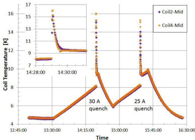
Fig. 5. Coil temperature rise due to background heat load when PTCC is turned off with magnet powered at fixed currents; rapid temperature rise and recovery (insert) from eddy current heating due to fast current discharge into dump resistor.
