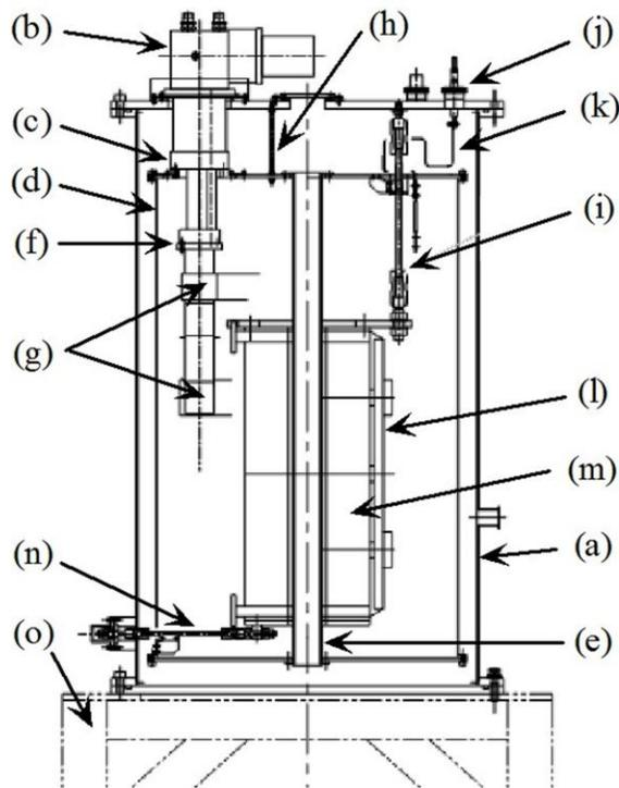
Fig. 1. Conduction cooling test stand assembly: a) vacuum vessel, b) pulse-tube cryo cooler, c) PTCC 1<sup>st</sup> stage, d) radiation shield, e) warm bore tube, f) PTCC 2<sup>nd</sup> stage, g) Pure Al, Cu connection bars, h) shield support, i) magnet support, j) hermetic feed through, k) copper lead, l) conduction cooling block, m) splittable quadrupole magnet, n) horizontal support, o) stand.
