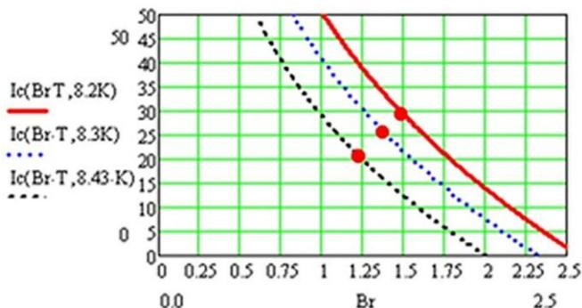
Fig. 6. The superconductor critical current as a function of coil peak field. Dots represent the quench currents (20 A, 25 A, 30 A) at elevated coil temperatures (8.43 K, 8.3 K, 8.2 K).
