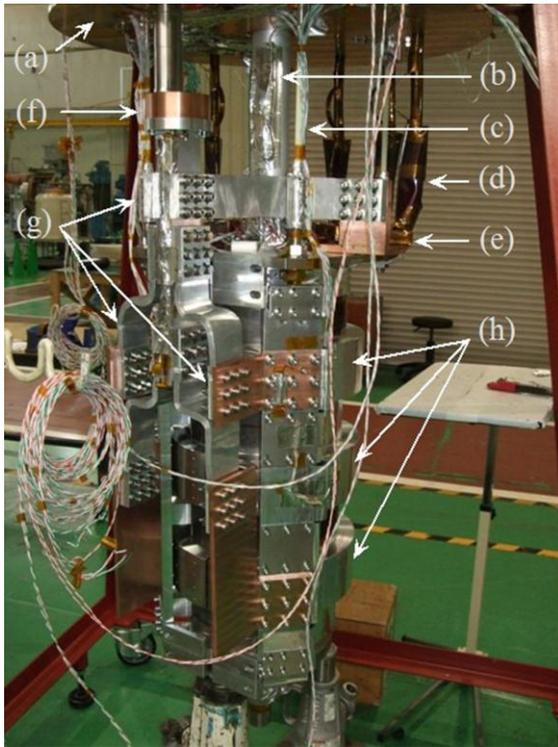
Fig. 3. Conduction cooling test stand during construction: a) top radiation shield, b) warm bore shield, c) vertical magnet support, d) Cu lead below HTS, e) Cu/SC lead thermal anchor, f) PTCC stage 2 cold head, g) pure Al and Cu conduction channels, h) stainless steel clamps around magnet yoke.
