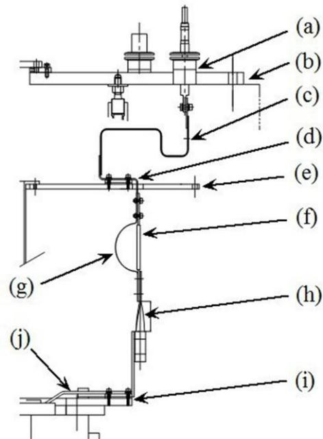
Fig. 2. Current Lead Construction: a) ceramic power feed-through, b) Vacuum vessel top plate, c) Copper lead, d) 50 K thermal anchor, e) radiation shield, f) HTS lead, g) Stainless Steel bypass lead, h) Flexible Copper lead, i) Copper Lead 4K thermal anchor, j) Copper-stabilized NbTi lead.
