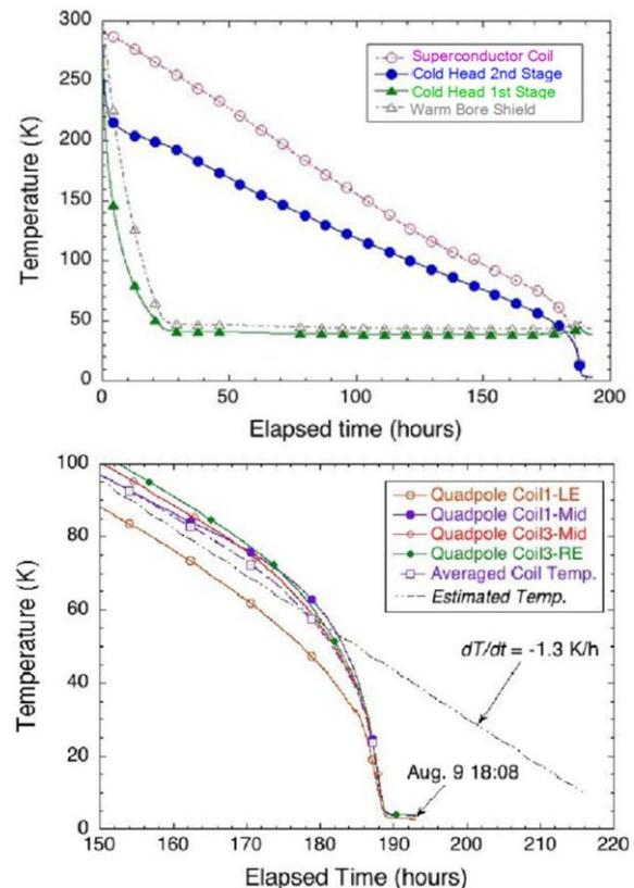
Fig. 4. Cool down from 300 K to 4 K (top), detail of final cooling phase from 40 K to 4 K (bottom).
