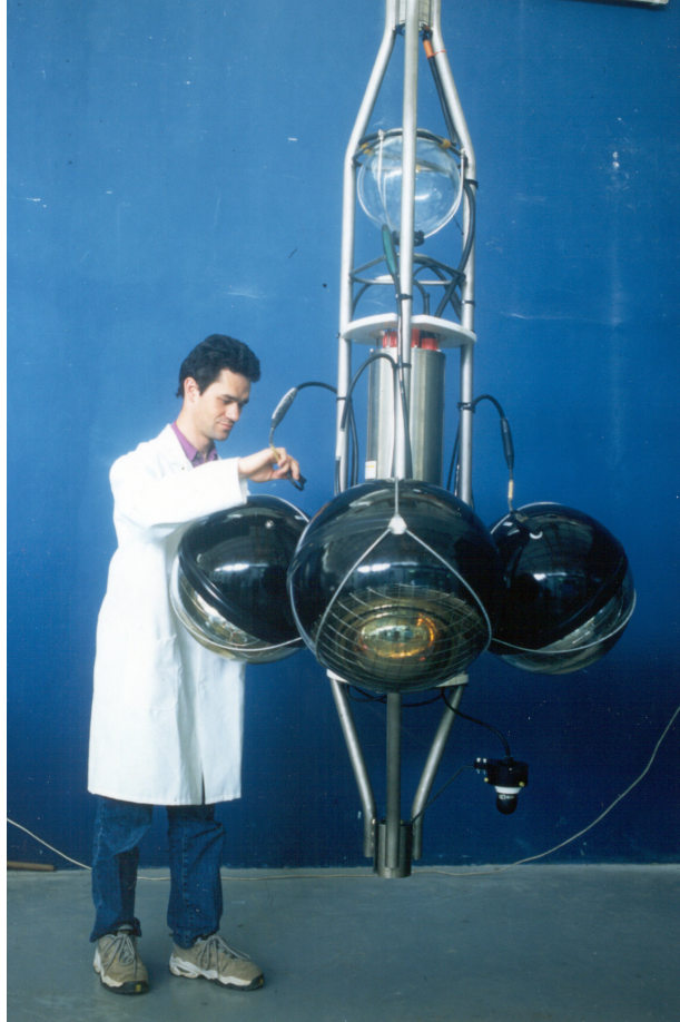
Figure 3.3: Detailed view on a storey with its three optical modules
