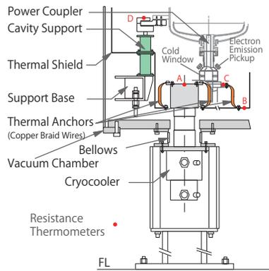
Figure 7: Schematic of the thermal shield showing thermometers and thermal anchors.
