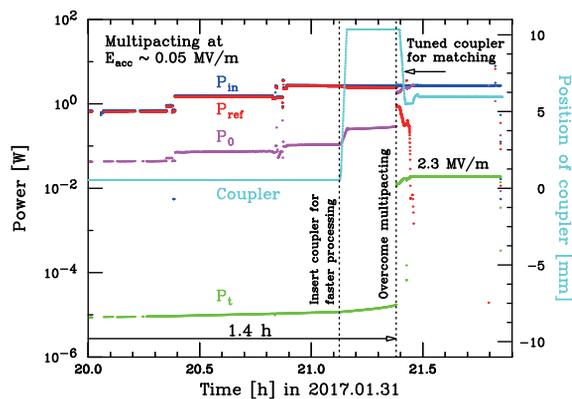
Figure 5: Demonstration of multipacting conditioning during VT4.
