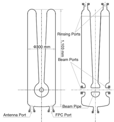
Figure 8: Schematic of the prototype 73-MHz cavity for vertical tests.
