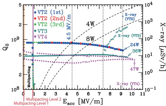
Figure 4:  $Q_0$  as a function of  $E_{acc}$  for vertical tests 2, 3, and 4.
