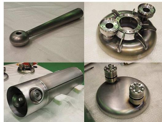
Figure 9: Niobium subassemblies for the prototype.
