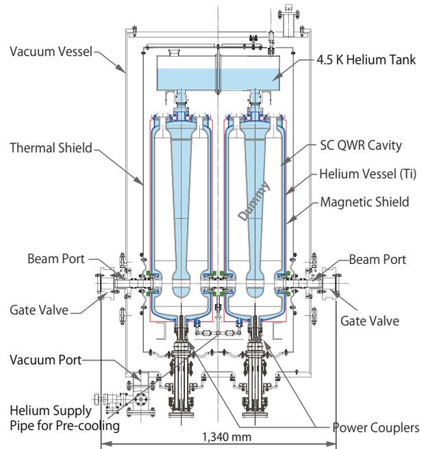
Figure 6: Schematic of the prototype cryomodule.
