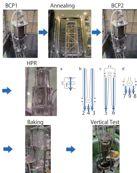
Figure 2: Procedure for surface treatment.
