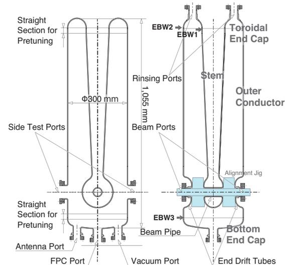
Figure 1: Schematic of the prototype QWR cavity (75.5 MHz).
