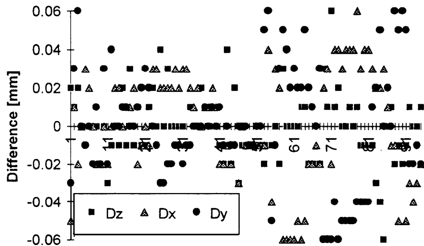
Fig. 18 Coordinate Differences between two Surveys with same Geometry
