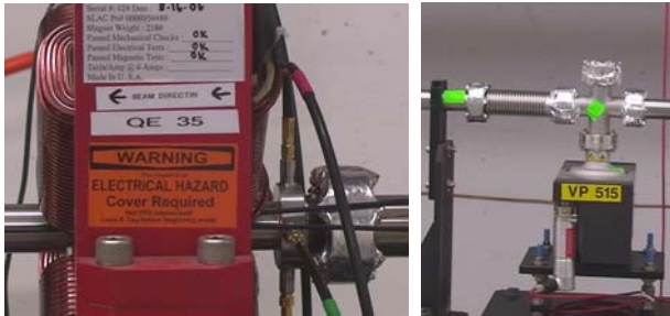
Figure 3: LTU strip-line BPM. “Lesker” bellows and a vacuum cross.
