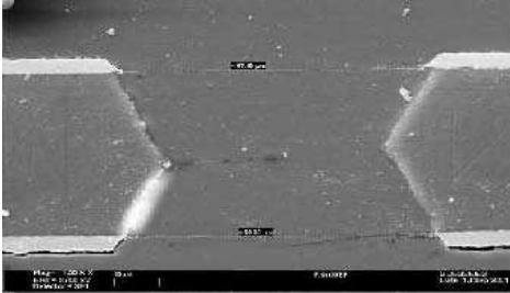
Figure 3.9: Picture of a GEM hole cross-section. The bi-conical profile of the hole is clearly visible [41].
