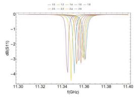
Figure 5: The reflection coefficient curves of the cavity model with different values of the relative permeability.
