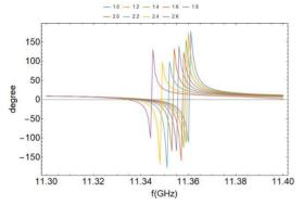
Figure 6: The phase curves of the cavity model with different values of the relative permeability.
