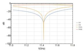
Figure 3: The simulated S-parameters of the revised RF polarizer with the resonant frequency of 11.424 GHz.
