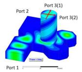
Figure 2: The simulation model of the revised RF polarizer.
