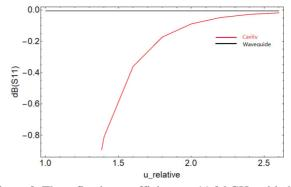
Figure 8: The reflection coefficients at 11.36 GHz with different  $\mu$  values.
