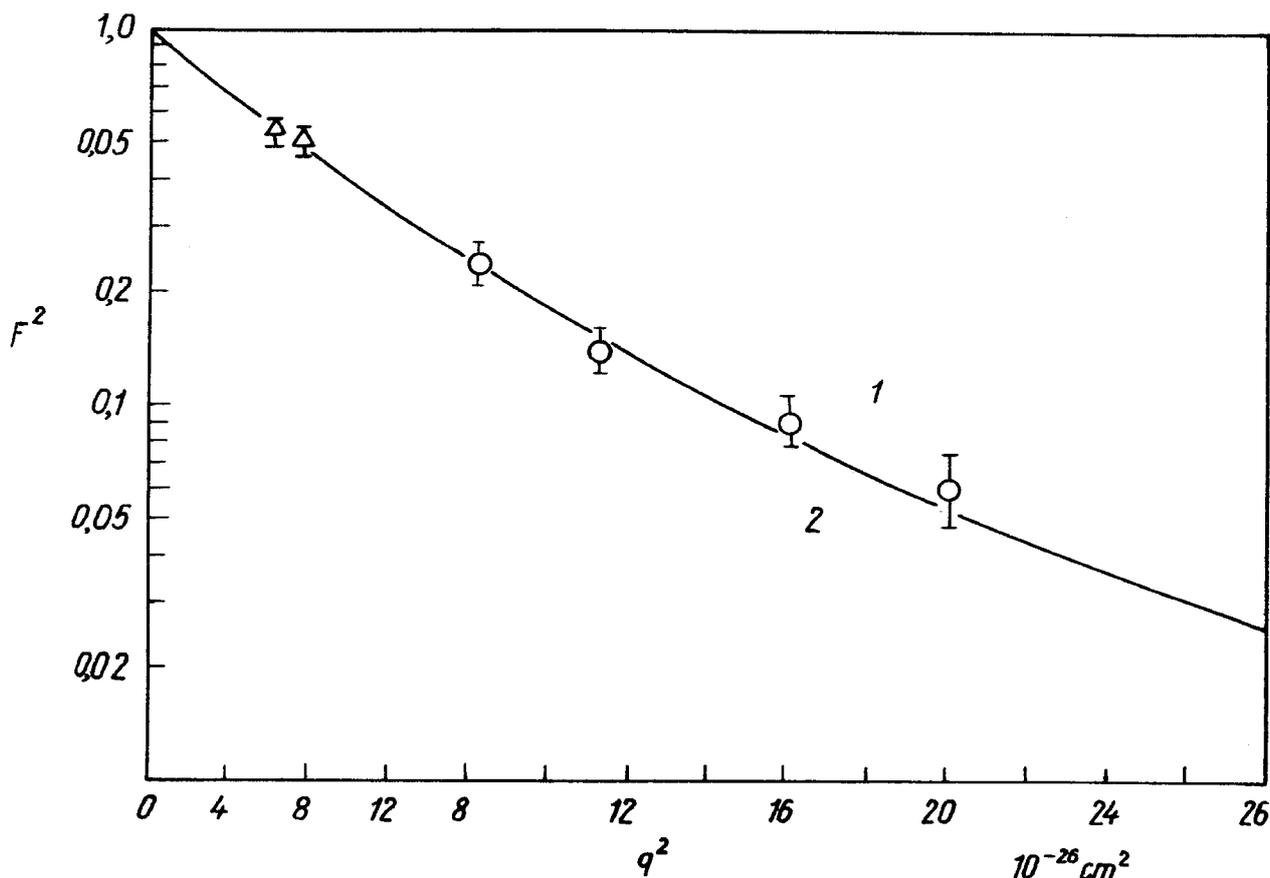
Fig.13. The square of the proton form factor (electric and magnetic assumed equal) as obtained from electron scattering from the internal beam of the 1.2 Bev Cornell synchrotron. The solid curve corresponds to an exponential model of 0.8 fermi RMS radius, 1 corresponds to  $a = 0.7$  fermi, 2 corresponds to  $a = 0.9$  fermi.
