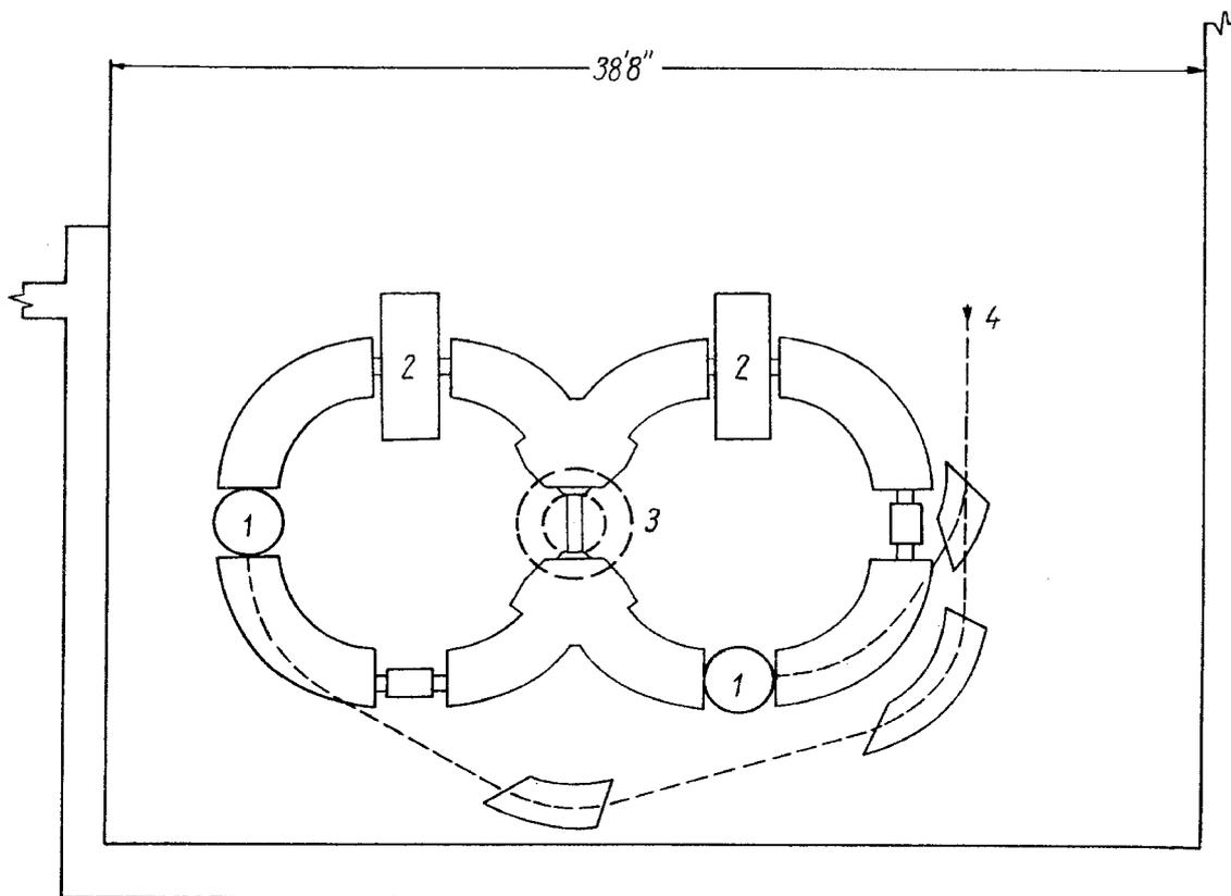
Fig.1. Diagram of electron-electron colliding beam experiment at Stanford University. 1 - the pulsed, inflector; 2 - R.F.cavities; 3 - interaction region; 4 - the incident beam.
