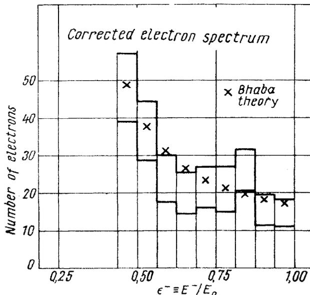
Fig.4. Experimental results of Poirier, Bernstein and Pine on electron-positron scattering at 200 Mev. Lower and upper experimental limits are shown as well as the values calculated from Bhabha theory.
