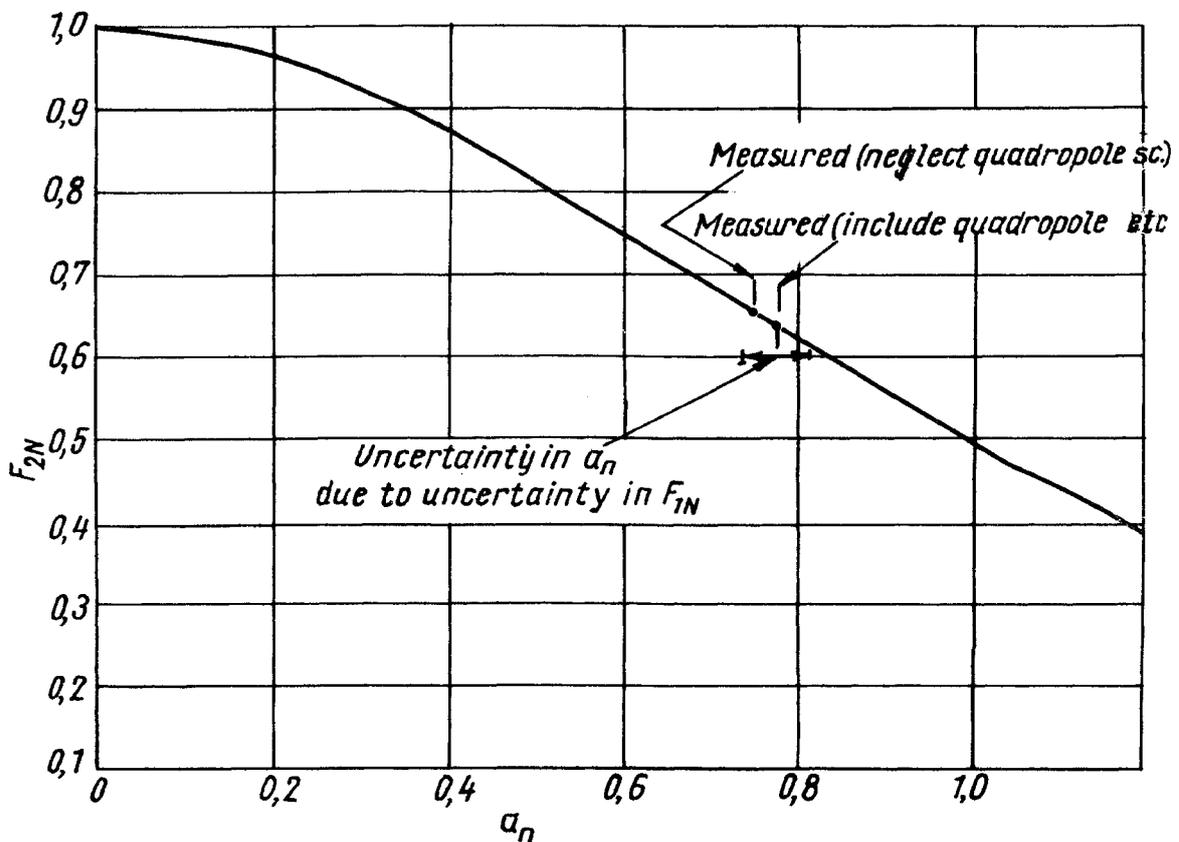
**Fig. 10.** The form factor curve of the magnetic moment distribution of the neutron as determined by elastic electron scattering  $E_0 = 260$  Mev  $\theta = 145^\circ$ . Contributions from quadropole scattering and an assumed neutron charge distribution are indicated:
