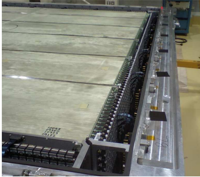
Figure 1.12: View of FGD with its scintillator bar modules stacked. (Original in colour.)
