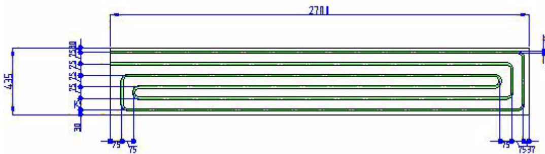
Figure 3-6 Cold plate pipes schematic
