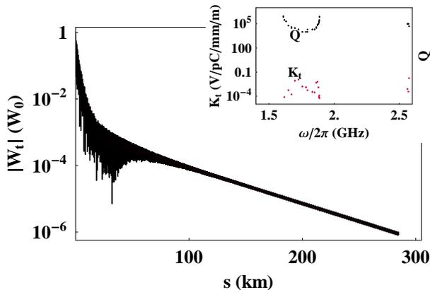
Fig. 2: Envelope of TESLA transverse wakefield. The abscissa runs over the distance of the complete bunch train. The ordinate has been normalised with respect to  $W_0$ , (0.11V/pC/mm/m). The kick factors and Q values are shown in the inset.
