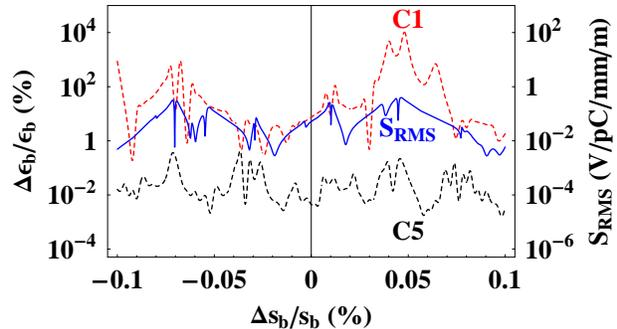
Fig. 3: Emittance dilution,  $\Delta\epsilon/\epsilon$ , for a single class of cavities (C1 shown in red) and for five classes of cavities (C5 shown in black). The RMS of the sum wakefield,  $S_{RMS}$ , is also illustrated for a single class of cavities (shown in blue)
