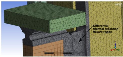
Figure 3: FEA Mesh - Flexure region has a 2 mm mesh.
