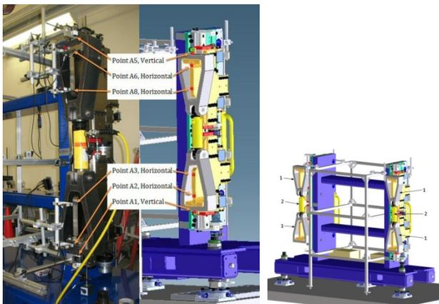
Figure 8: Keyence sensors, shown in the photo on the right, were mounted onto the external frame and touching the flexure plates. The second image shows the gap drive test plates.
