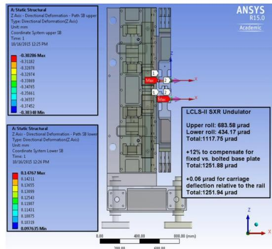
Figure 7: Combined results of the roll between the upper and lower strongbacks.
