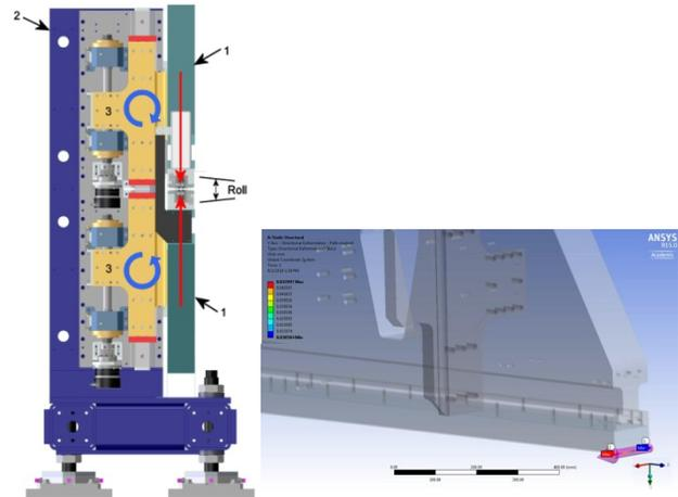
Figure 6: Left image is an end view of undulator showing the drive assemblies. Right image is the FEA analysis result showing the path used to calculate the roll.
