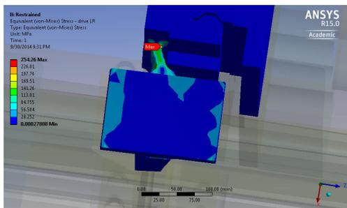
Figure 4: Close-up of the maximum stress of 254 MPa at a temperature of 5°C, located in the lower flexure plate.
