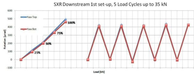
Figure 9: Measured roll of the prototype SXR. The maximum load is 35 kN, which corresponds to the gap drive load for the SXR.
