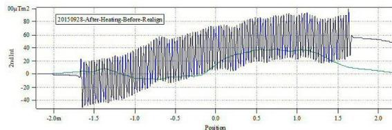
Figure 5: Plot of the second field integrals (trajectories) before and after a thermal cycle from 20°C to 35°C and back.
