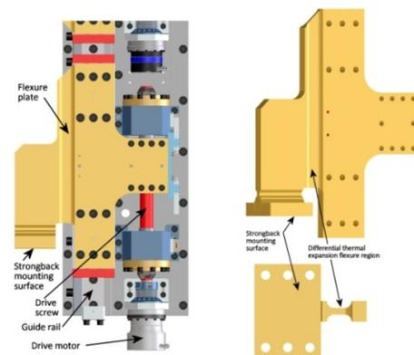
Figure 2: Front view of flexure plate mounted on a bottom drive. The flexure region on each flexure plate allows for differential thermal expansion/contraction between the steel frame and the aluminium strongbacks.
