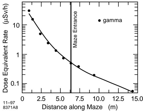
Figure 5: Dose Equivalent as a Function of Distance along Maze for  $^{137}\text{Cs}$
