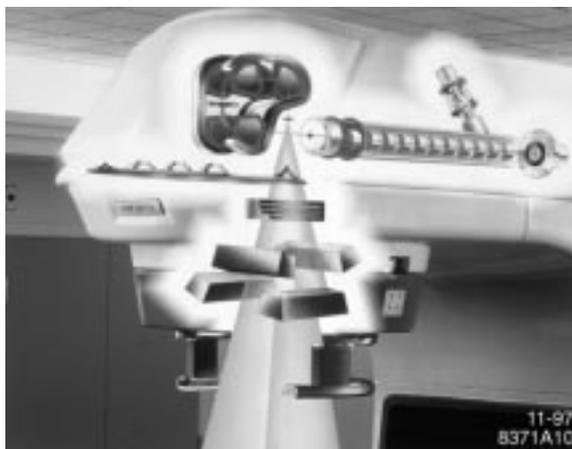
Figure 1: Schematic of a Medical Accelerator Head
