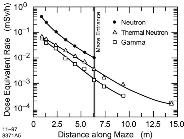
Figure 4: Dose Equivalent as a Function of Distance along Maze for W- Moderated  $^{252}\text{Cf}$
