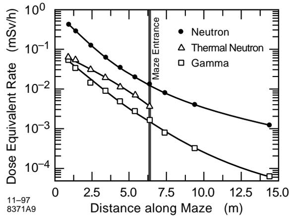
Figure 3: Dose Equivalent as a Function of Distance along Maze for  $^{252}\text{Cf}$
