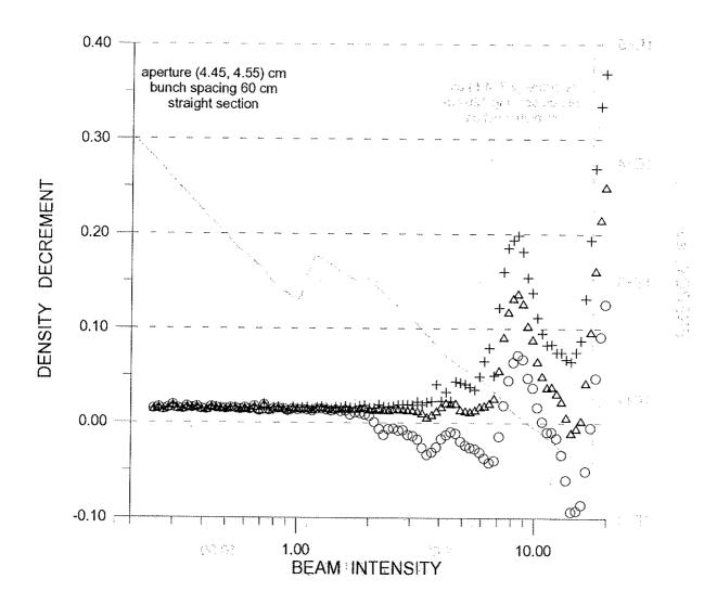
Figure 4: Same spacings as previous, but the chamber is round. The yield constants  $\hat{\eta}$  are 1.1, 1.4 and 1.8 marked by +,  $\triangle$  and o.
