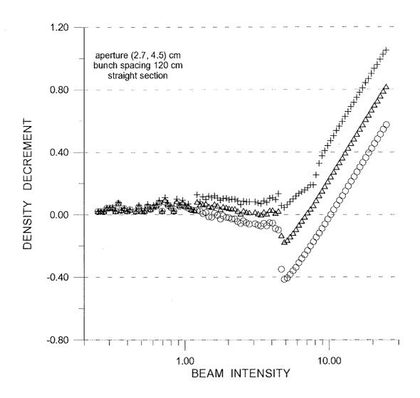
Figure 1: Electron density decay rate for various secondary emission yield constants  $\hat{\eta}$ : 1.1, 1.4 and 1.8, labeled by +,  $\triangle$  and  $\circ$  correspondingly. The vacuum chamber and beam separations are taken as PEP-II.
