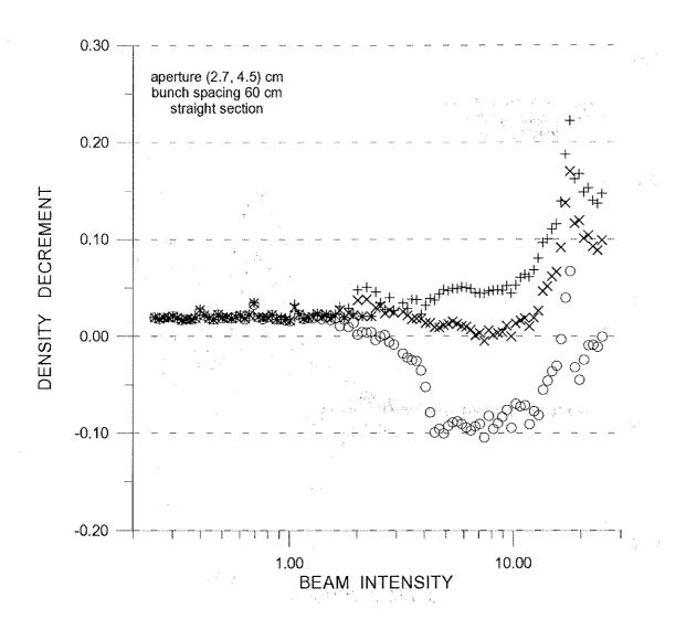
Figure 3: The chamber and spacings are for KEKB project. The yield constants  $\hat{\eta}$  are 1.1, 1.3 and 1.8 marked by +, × and  $\circ$ .
