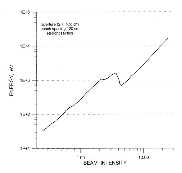
Figure 5: Average electron energy as a function of beam current for the PEP-II parameters.
