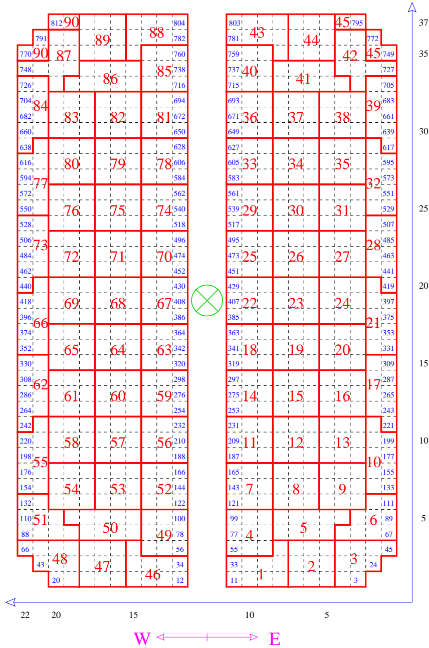
Figure 3.7: Schematic view of the Inner Electromagnetic calorimeter as seen by the beam. The thin dashed lines show each lead glass block; the thick solid lines show the blocks which make up each sum. All numbers are part of the internal numbering schemes. Sums 1–15 compose the first sextant of the dielectron trigger, sums 16–30 compose the second sextant, etc.
