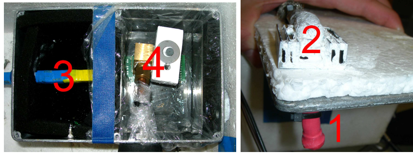
Figure 2.3: Photo of the open box (left) and the cover (right): 1- G-MAPD with shielding , 2- pre-amplifier wrapped in a shielding in thermal contact with a heat-exchanger, 3- light conductor , 4- automatic level control valve inside the bath for the cryogenic liquids.
