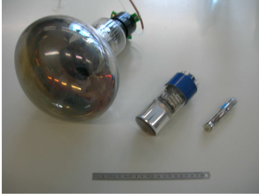
Figure 1.3: Three PMTs of different size next to a 20 cm long ruler: the Hamamatsu R5912-02MOD used in the medium LAr TPC experiment at LHEP Bern (left), the Philips 53AVP which is similar in size to the Hamamatsu R7725 MOD (middle), the Hamamatsu R1450 used for some test runs in the small LAr TPC (right).
