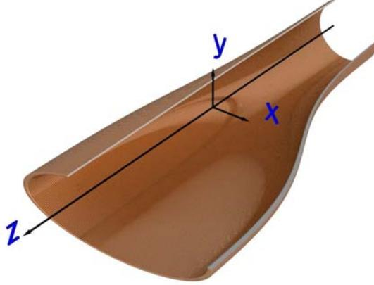
FIG. 1: A smooth transition of a beam pipe (a cutaway drawing shows the interior part of the pipe).
