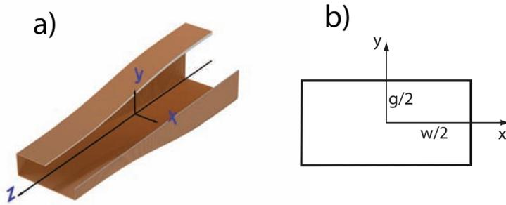
FIG. 3: A smooth transition with rectangular cross section, *a*); the origin of the coordinates  $(x, y)$  is located at the center of the rectangle, *b*).
