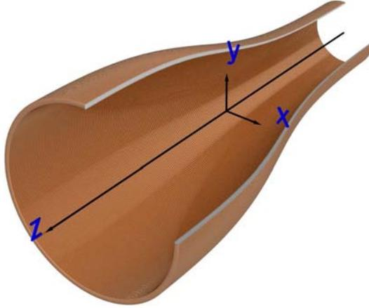
FIG. 2: Geometry of a round transition.
