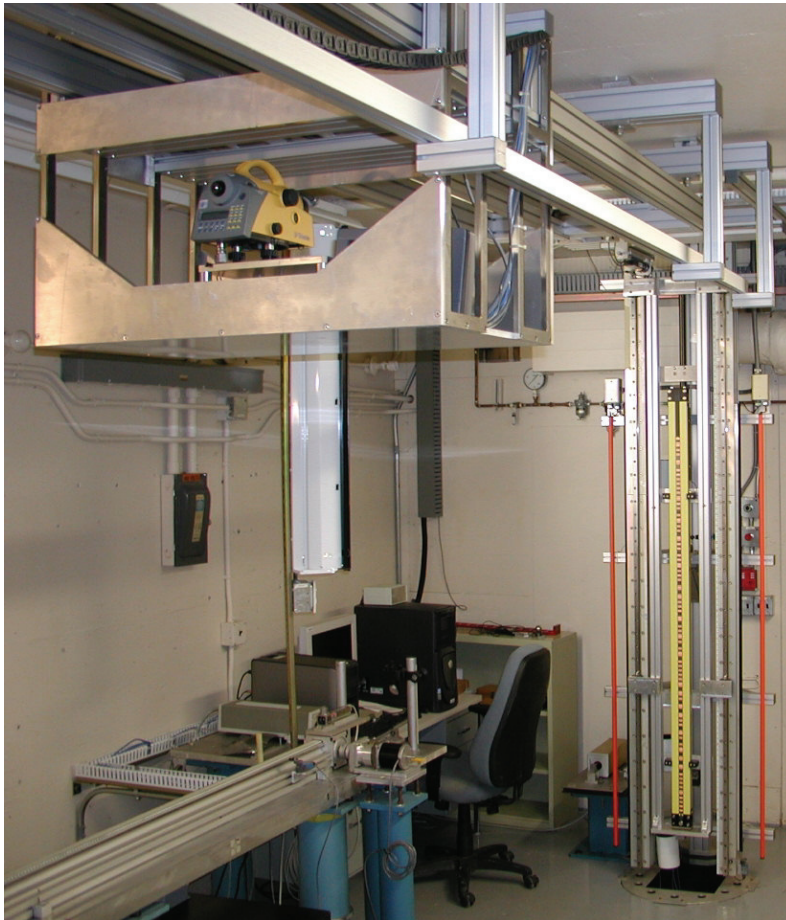
Figure 2: Overview of the vertical comparator.
