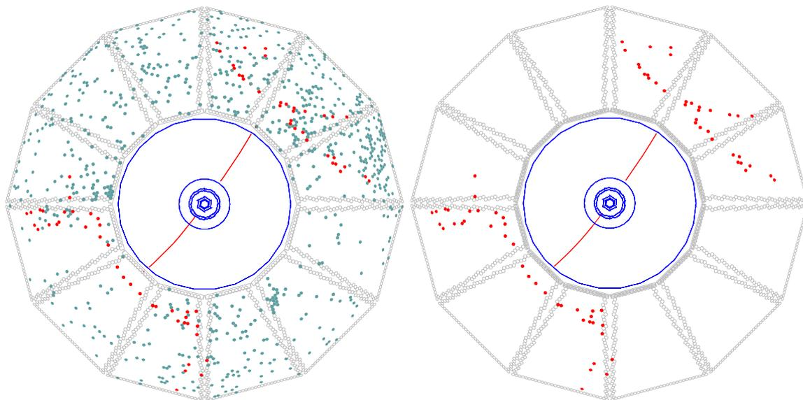
Figure 3.14: Display of an  $e^+e^- \rightarrow \mu^+\mu^-$  event reconstructed in *BABAR* with two different time cuts. On the left, all DIRC PMTs with signals within the  $\pm 300$  ns trigger window are shown. On the right, only those PMTs with signals within 8 ns of the expected Čerenkov photon arrival time are displayed.
