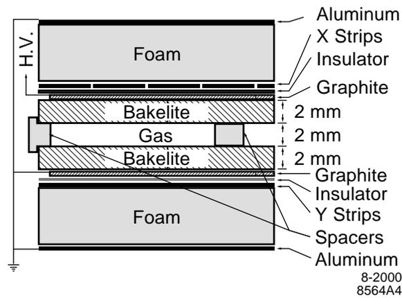
Figure 3.18: Cross-section of a *BABAR* RPC.
