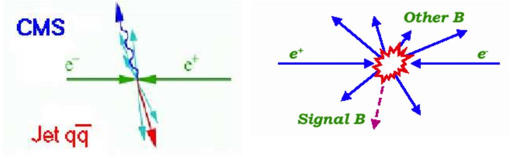
Figure 2.2: Schematic topological representations of (left)  $e^+e^- \rightarrow q\bar{q}$  and (right)  $e^+e^- \rightarrow \Upsilon(4S) \rightarrow B\bar{B}$  events.
