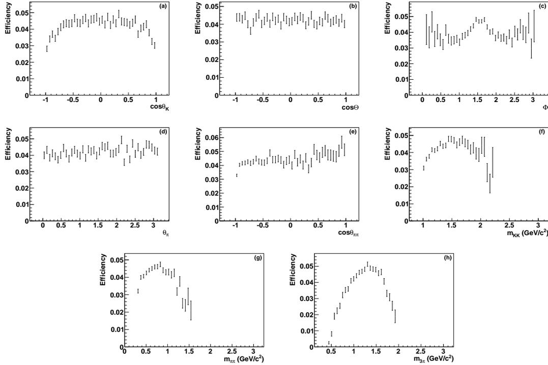
Figure 4.33: 1D projections of  $\gamma\gamma \rightarrow \eta_c(1S) \rightarrow K^+ K^- \pi^+ \pi^- \pi^0$  efficiency on (a)  $\cos \theta_K$ , (b)  $\cos \Theta$ , (c)  $\Phi$ , (d)  $\theta_\pi$ , (e)  $\cos \theta_{\pi\pi}$ , (f)  $m_{KK}$ , (g)  $m_{\pi\pi}$ , and (h)  $m_{3\pi}$ .
