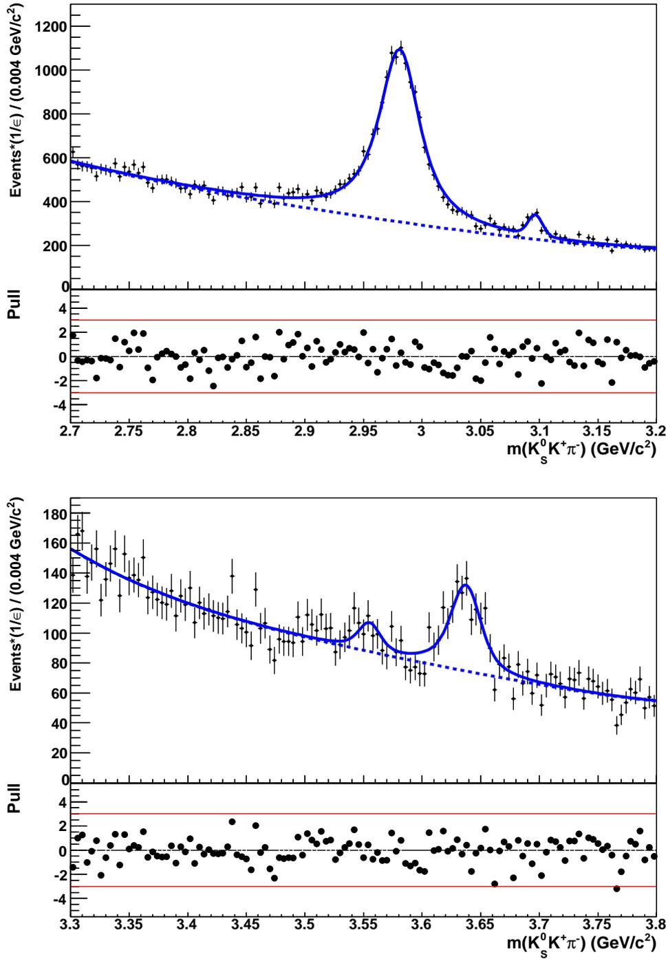
Figure 4.38: Fit to the  $K_s^0 K^\pm \pi^\mp$  efficiency-weighted mass spectrum in the (a)  $\eta_c(1S)$  region and (b)  $\eta_c(2S)$  region. The solid line is the total fit function, the dashed line is the background component. In each plot we also show the distribution of the error-normalized difference (pull) between the fit function and the data points.
