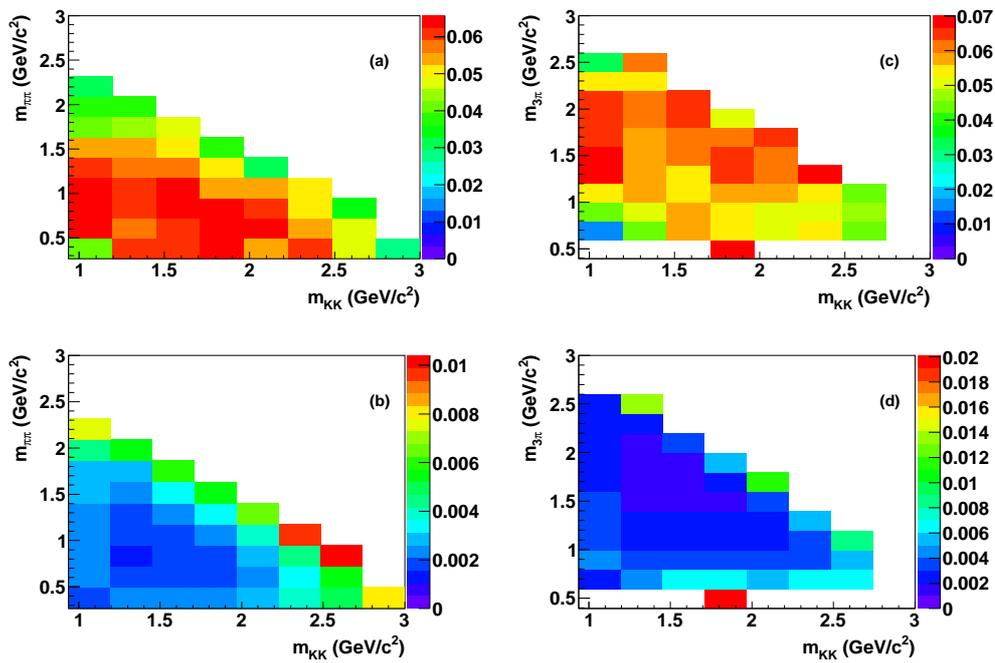
Figure 4.36: Signal efficiency ((a) and (c)), and its uncertainty ((b) and (d)) distributions over the  $(m(KK), m(\pi\pi))$  and  $(m(KK), m(3\pi))$  planes, for the  $K^+ K^- \pi^+ \pi^- \pi^0$  decay mode in the  $\eta_c(2S)$  mass region.
