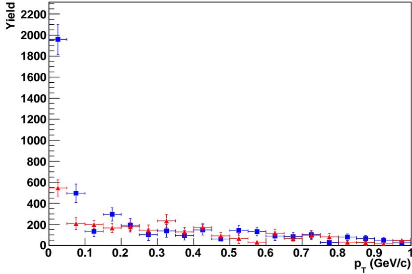
Figure 4.12: Distribution of the  $\eta_c(1S)$  (blue squares) and  $J/\psi$  (red triangles) yield extracted from a fit to the  $K^+K^-\pi^+\pi^-$  invariant mass spectrum. Results are reported in different  $p_T$  intervals.
