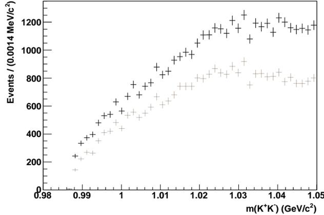
Figure 4.21: Mass distribution for  $\pi^+\pi^-$ , when assigning kaon mass hypothesis to the pion. In the black only requirements described in sec. 4.4.3 are applied. In the grey plot we further require  $-0.5 < \cos\theta_{\pi^+}^H < 0.5$ .
