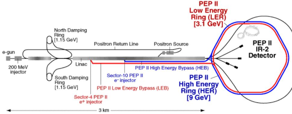
Figure 3.3: The PEP-II asymmetric storage ring and the SLAC linear accelerator. The SLAC linac is the injector for PEP-II. The single interaction point of PEP-II is at Interaction Region 2, where *BABAR* is situated.
