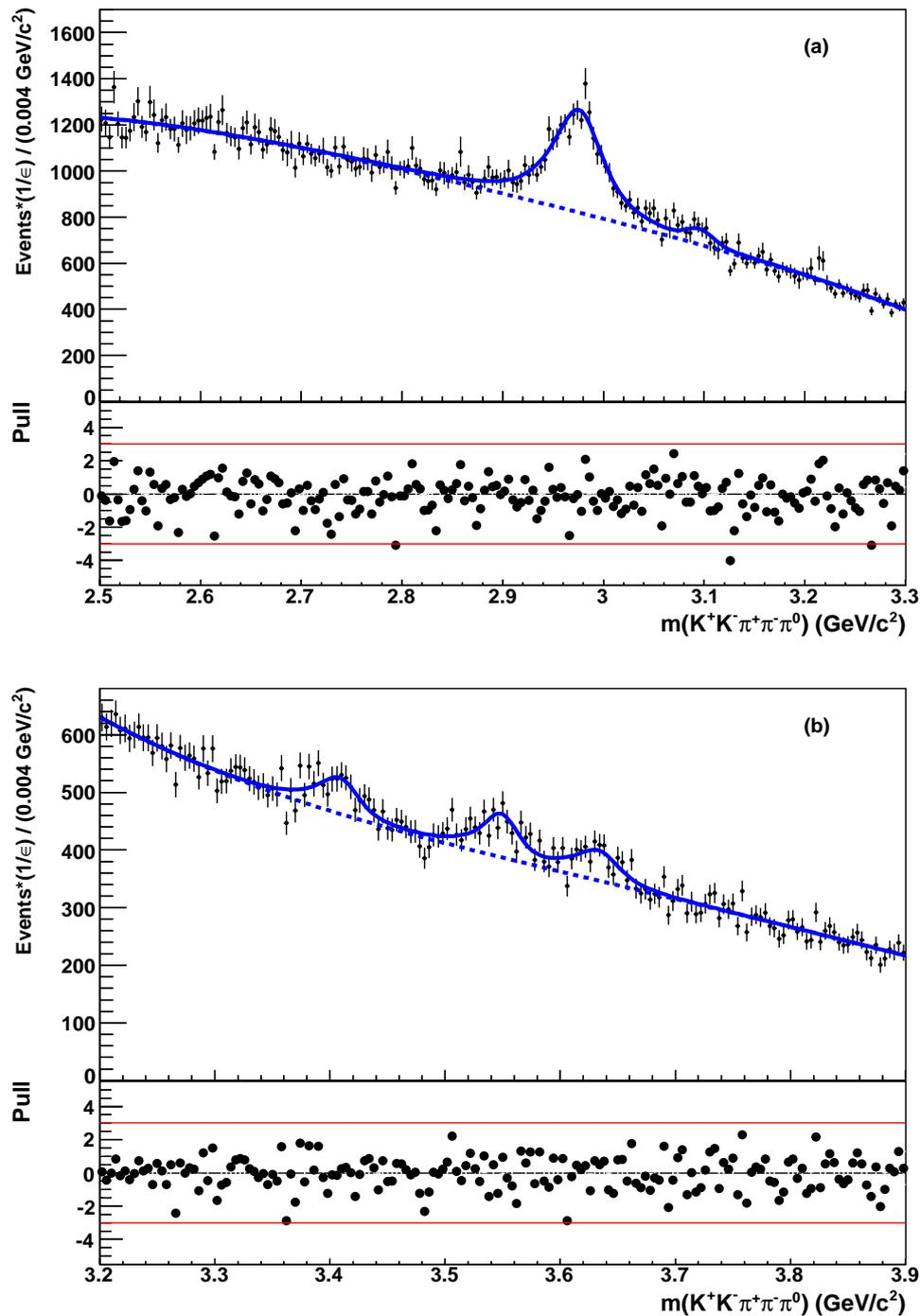
Figure 4.39: Fit to the  $K^+K^-\pi^+\pi^-\pi^0$  efficiency-weighted mass spectrum in the (a)  $\eta_c(1S)$  region and (b)  $\eta_c(2S)$  region. The solid line is the total fit function, the dashed line is the background component. In each plot we also show the distribution of the error-normalized difference (pull) between the fit function and the data points.
