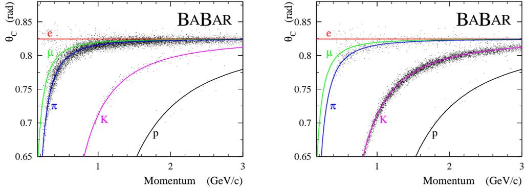
Figure 3.15: Čerenkov angle distributions, as a function of the momentum, for (left)  $\pi$  and (right)  $K$  events from control sample. The control sample used is  $D^{*+} \rightarrow D^0 (\rightarrow K^- \pi^+) \pi^+$ .
