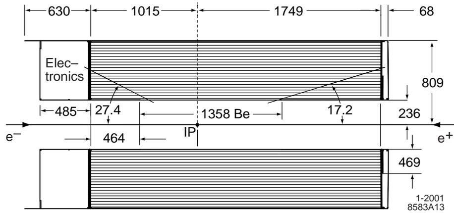
Figure 3.9: Longitudinal section of the drift chamber.
