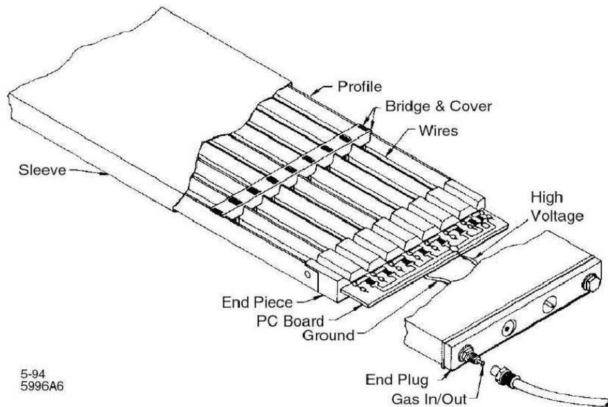
Figure 3.20: Diagram of a prototypical limited streamer tube.
