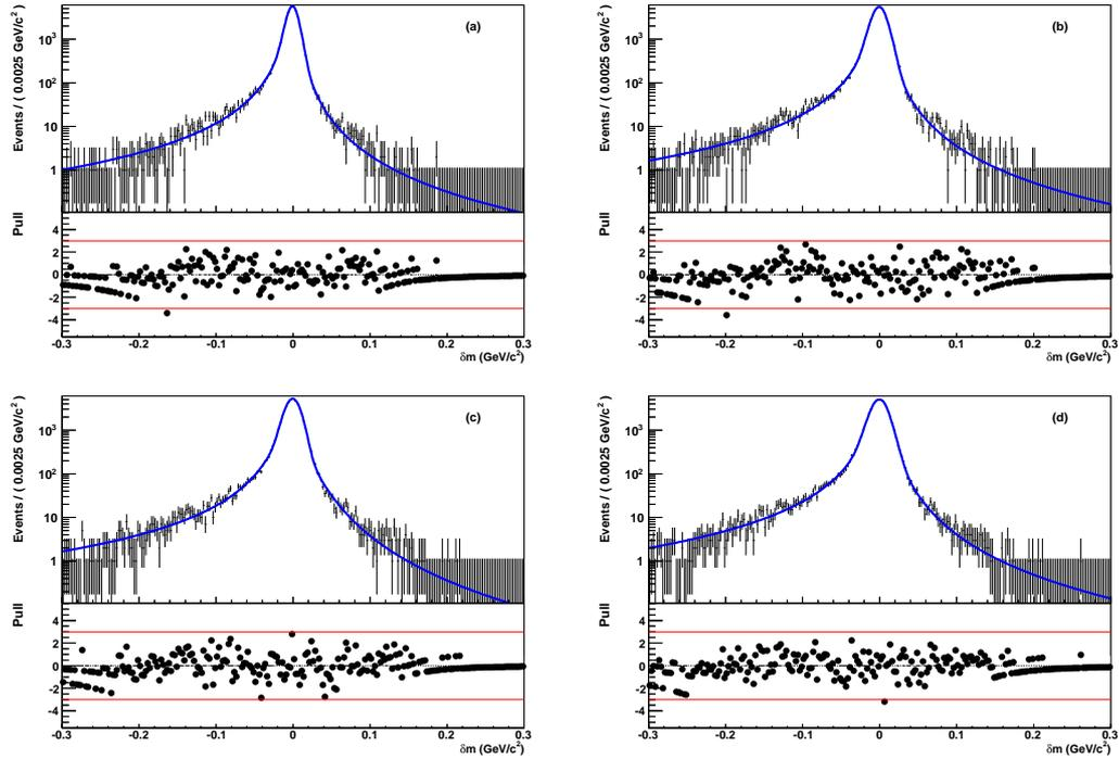
Figure 4.23: Distribution of  $\delta m$  (a)  $\eta_c(1S)$ , (b)  $\chi_{c2}(1P)$ , (c)  $\eta_c(2S)$ , and (d)  $\chi_{c2}(2P)$  MCT events, in  $K_s^0 K^\pm \pi^\mp$  decay mode. The blue solid curve is the fit function (see text for details). In each figure we also show the distribution of the error-normalized difference (pull) between the fit function and the data points.
