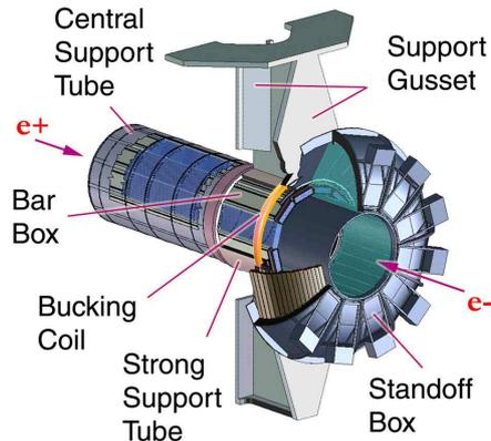
Figure 3.12: View of the DIRC mechanical structure.
