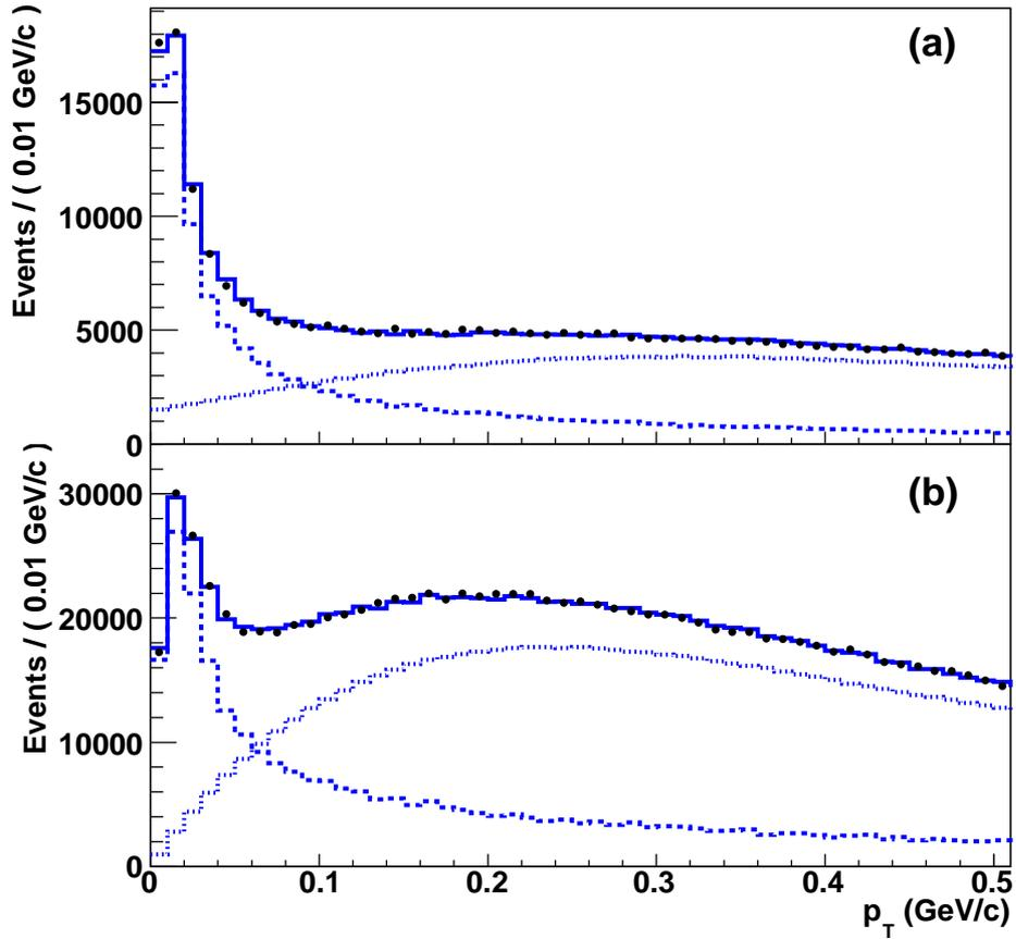
Figure 4.10: The  $p_T$  distributions for selected (a)  $K_s^0 K^\pm \pi^\mp$  and (b)  $K^+ K^- \pi^+ \pi^- \pi^0$  candidates (data points). The solid histogram represents the result of a fit to the sum of the simulated signal (dashed) and background (dotted) contributions. Figure published in Ref. [324]
