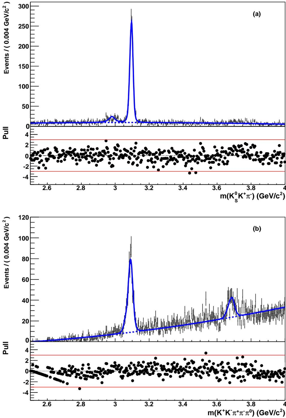
Figure 4.26: Fit to (a)  $K_S^0 K^\pm \pi^\mp$  and (b)  $K^+ K^- \pi^+ \pi^- \pi^0$  mass spectrum for real data satisfying the reversed  $M_{\text{miss}}^2$  requirement (see text). The solid line is the total fit function, the dashed line is the background component. In each plot we also show the distribution of the error-normalized difference (pull) between the fit function and the data points.
