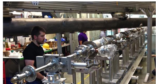
Fig. 4. Left: Vacuum Vessel as received by Cornell University. Right: Marriage step: the cavity string coming from the clean room assembly is rolled under the HGRP providing precision alignment.
