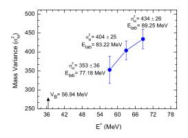
FIG. 1: Mass variance,  $\sigma_M^2$ , as a function of excitation energy  $(E^*)$  for deformed thulium target. The arrow indicates the  $E^*$  corresponding to the Coulomb barrier.
