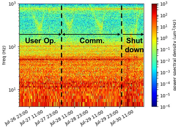
Figure 2: Power spectral density of vibration on optical table during 4 days.
