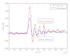
Figure 4: Typical waveforms from a charge amplifier with 50ns peaking time, measured with a digital oscilloscope at a sampling rate of 40MS/s and then interpolated. Note the asynchronous samples. This particular amplifier suffered from some ringing, but this is irrelevant to the measurement.
