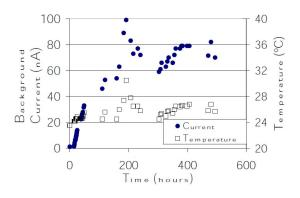
Figure 3: Evolution of the dark current as a function of time after the gas flow was reduced to 1 kg/year, at the nominal working voltage of 5600 V.
