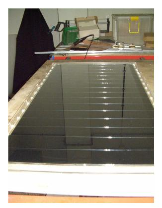
Figure 2: Double-gap RPC module with  $0.5 \times 1 \text{m}^2$ . The RPC is completely contained inside an impermeable high-voltage and gas enclosure.
