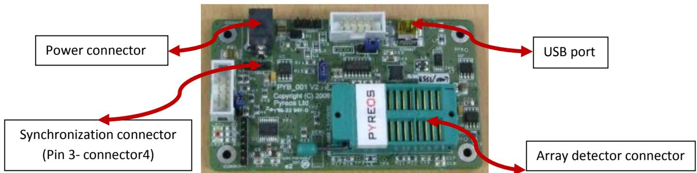
*Figure 2: Sensor PCD board.*
